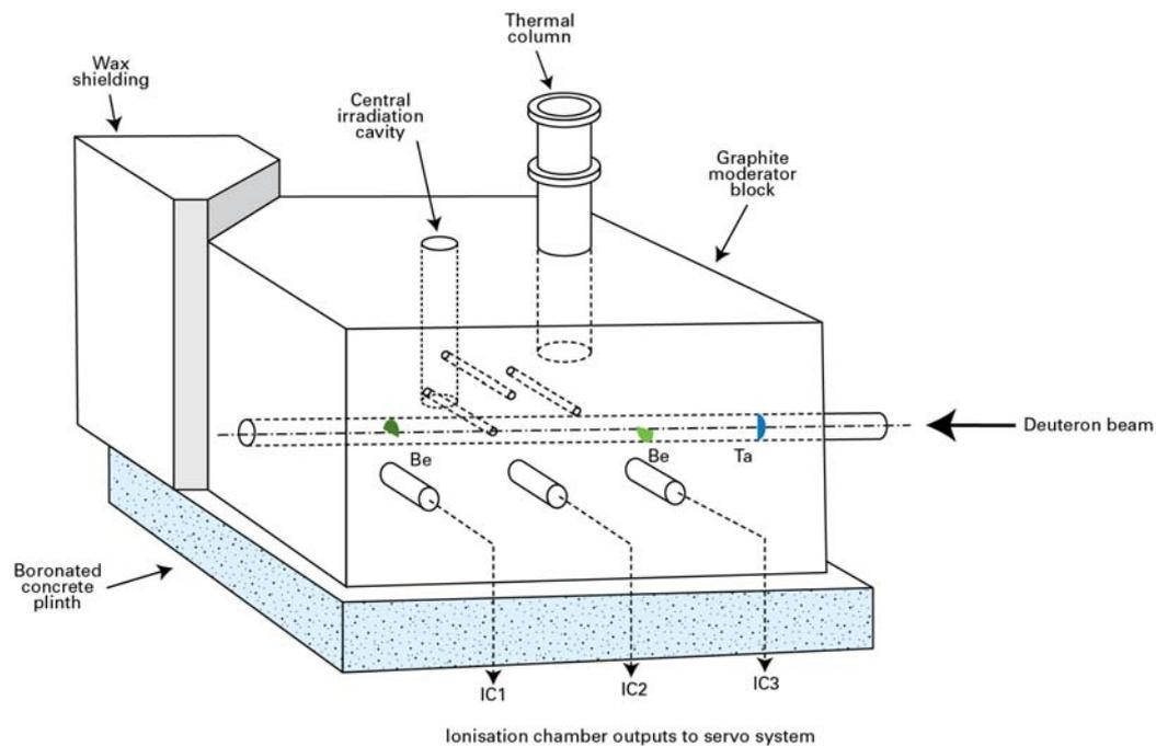
Figure 7. Schematic view of the NPL thermal pile
