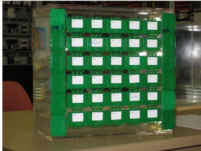
Figure 4. An ISO water phantom with the front face covered with passive personal dosimeters
