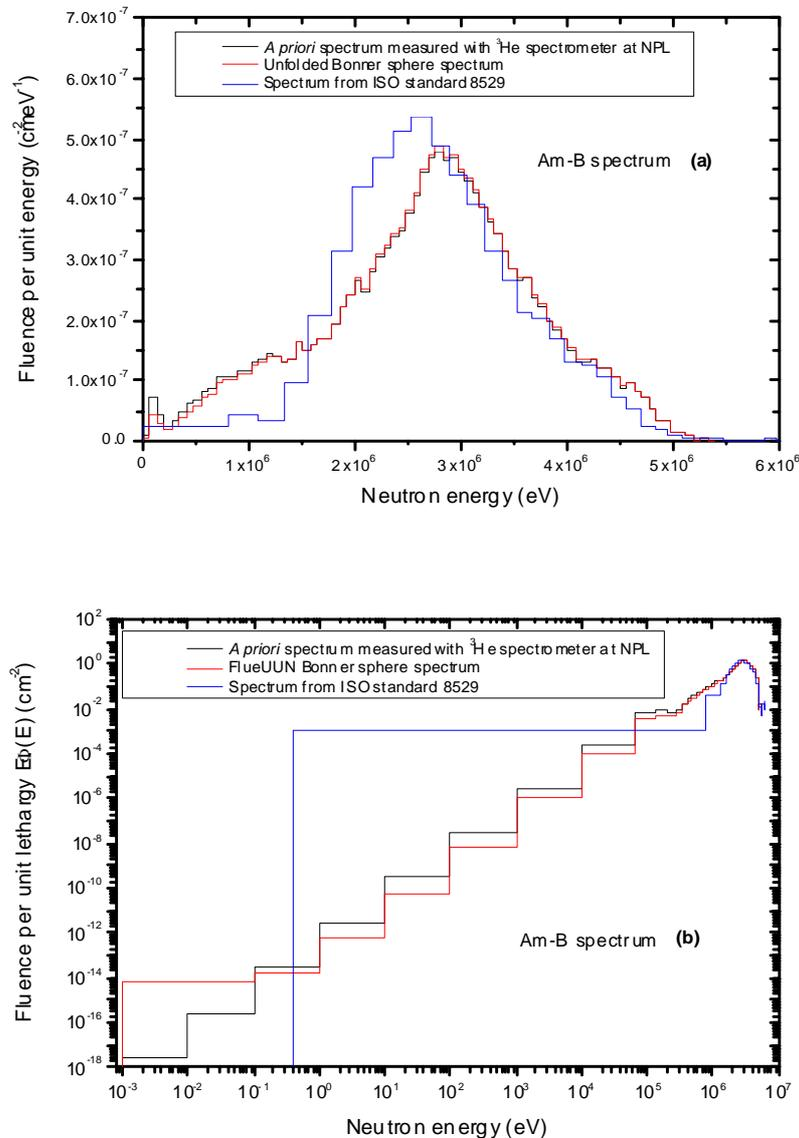
Figure 10. Results of Bonner sphere measurements of the  $^{241}\text{Am-B}$  spectrum showing the *a priori* information used for the unfolding, the unfolded spectrum, and the ISO recommended spectrum for this source.
