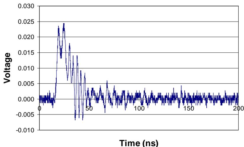
Figure 11. A typical linear pulse captured from the scintillation spectrometer.
