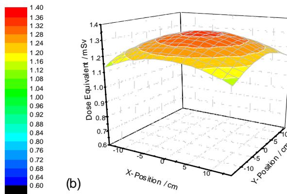
Figure 5. The top figure (a) shows the situation where the dose equivalent is assumed not to vary across the face of the phantom. It can be compared with the lower figure (b) where allowance has been made for all the effects which cause the dose equivalent to vary with position.
