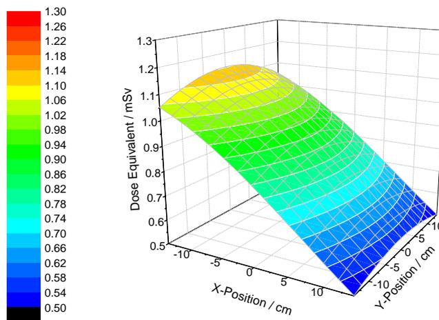
Figure 6. Variation of the dose equivalent across the surface of a phantom positioned at an angle of  $36^\circ$  to a charged particle beam producing 144 keV neutrons at  $0^\circ$  via the Li(p,n) reaction and 100 keV neutrons at  $36^\circ$ .
