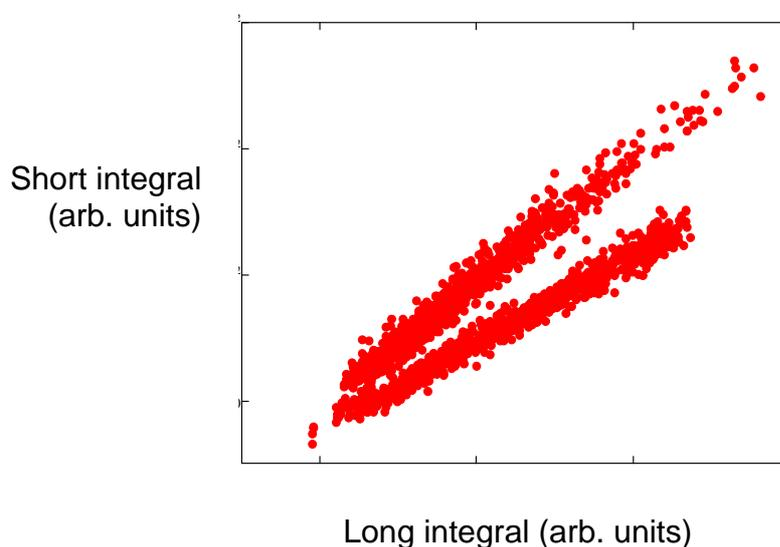
Figure 12. MathCAD plot showing Short vs. Long integrals for a number of spectrometer pulses (one dot per pulse). There is a clear separation into two populations, assumed to correspond to neutron events (upper branch) and gamma events (lower branch).
