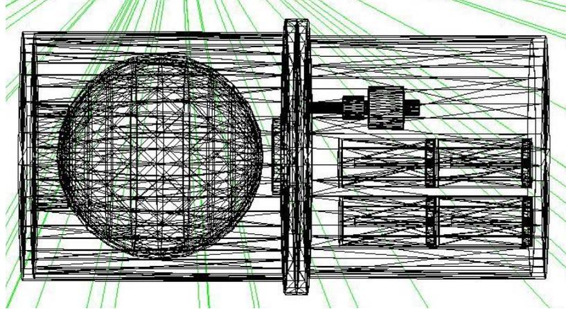
Figure 13 Wire mesh representation of the GEANT4 TEPC model illustrating the housing for the tissue-equivalent plastic sphere and support, 4x D cell batteries and gas filling valve. The green rays represent tracks from a neutron point source.
