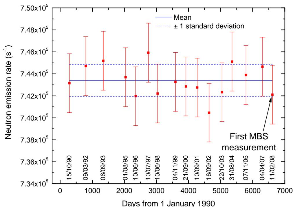
Figure 2: Annual measurements of the national standard  $^{226}\text{Ra-Be}$  source, decay corrected to 1 January 1990 (error bars correspond to only the random uncertainty components at  $1\sigma$ )
