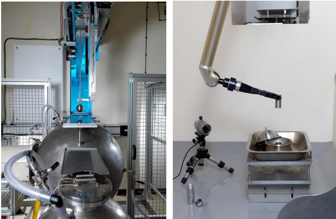
Figure 1: The source sphere being transferred into the large manganese bath (left), and source being loaded into the sphere using the manipulators in the source cell (right).
