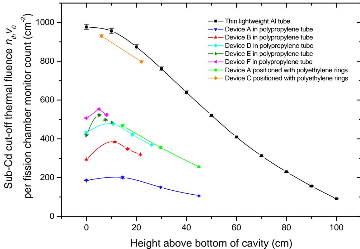
Figure 8. Variation of fluence per unit monitor count with height and type of device positioned in the central hole of the cavity
