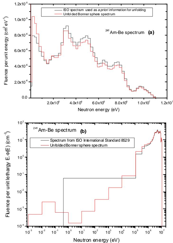
Figure 9. Results of Bonner sphere measurements of the  $^{241}\text{Am-Be}$  spectrum showing the ISO recommended spectrum used as *a priori* information for the unfolding, and the unfolded spectrum.
