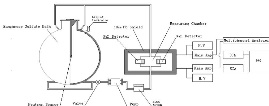
Fig.1. The manganese sulfate bath system
