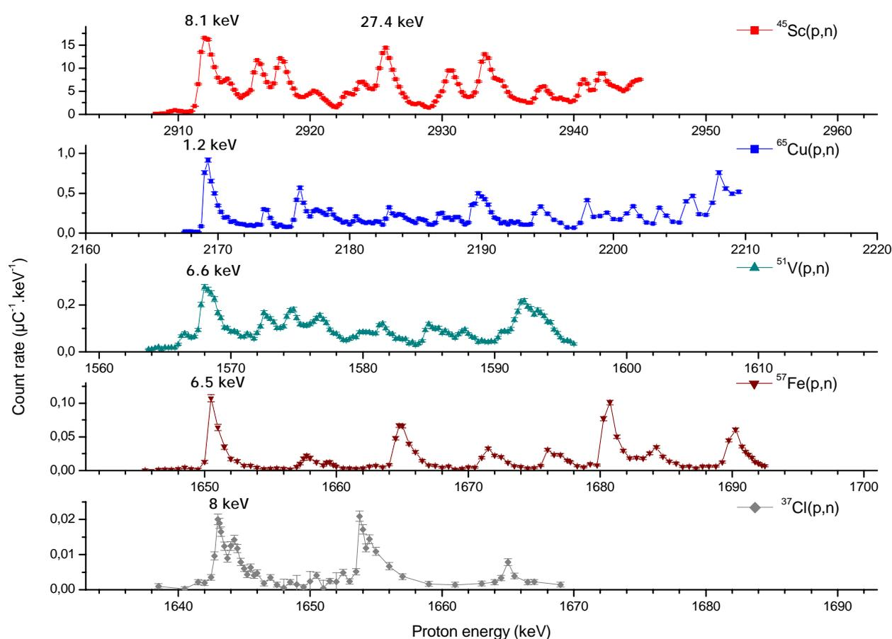
Figure 3: Count rate, for 1 keV ion beam energy loss in the target, for the IRSN long counter placed at  $0^\circ$  and 66 cm from the target for respectively  $^{45}\text{Sc}(p,n)$ ,  $^{65}\text{Cu}(p,n)$ ,  $^{51}\text{V}(p,n)$ ,  $^{57}\text{Fe}(p,n)$  and  $^{37}\text{Cl}(p,n)$  reactions, as a function of the proton beam energy.
