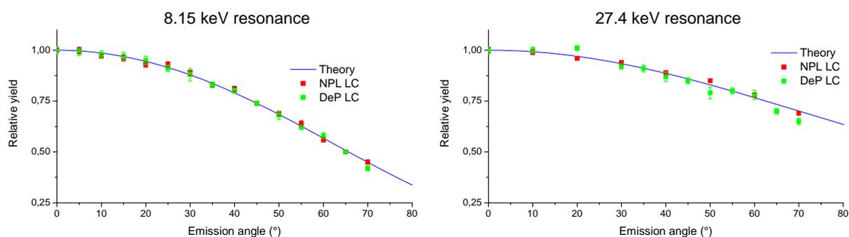
Figure 3: Variation of the neutron fluence, determined with two different long counters at NPL facility, as a function of the forward emission angle (up to  $70^\circ$ ) in the laboratory frame of reference, for the 8.15 and 27.4 keV resonances of the  $^{45}\text{Sc}(p,n)$  reaction and comparison with the theoretical variation in the case of an isotropic emission in the centre of mass.
