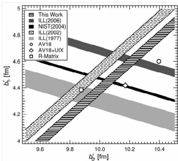
Figure 2: This work compared to previous experimental measurements on the  $n$ - $^3\text{He}$  system. Theoretical predictions are shown as single point.
