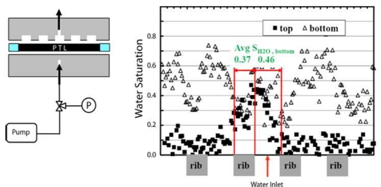
Figure 2: Left is the measurement device used in the experiment to mimic the compression of the PTL in a real fuel cell with channels and ribs. Right shows the measured water saturation as a function of position.
