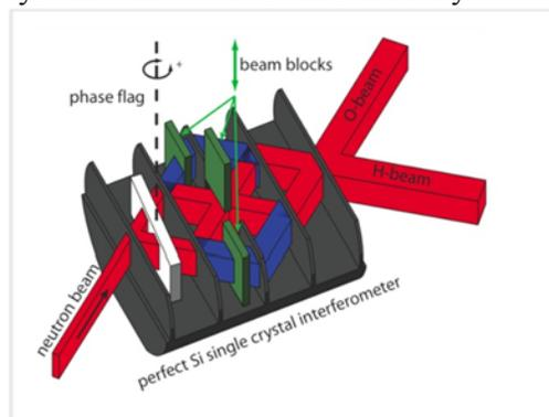
Figure 1: A schematic diagram of the 5-blade neutron interferometer. By changing the location of Cd beam blocks we can switch from a MZ and DF type interferometer without having to use completely different interferometer crystals.
