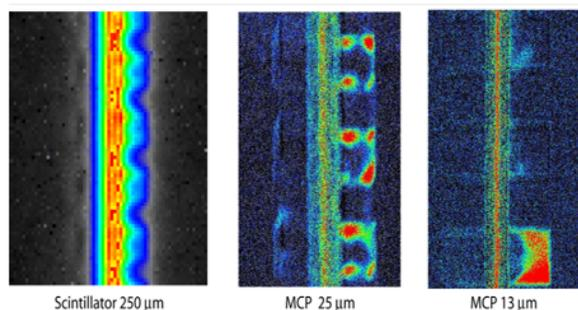
*Progression of improved spatial resolution in the measured through plane direction of a hydrogen fuel cell.*
