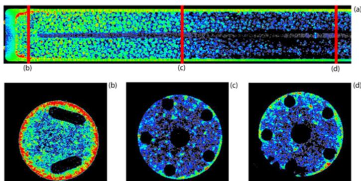
Figure 1. (a) Slice along the length of the storage bed, (b)-(d) axial slices from the locations denoted in (a).
