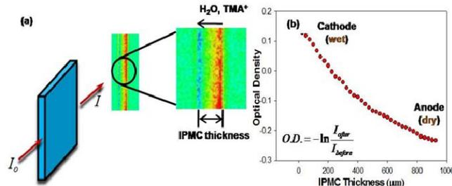
*Figure 2: (a) Colorized images showing water/counterion-depleted zones represented by red pixels and water/counterion-rich areas represented by blue pixels. IPMC was subjected to 3 VDC. (b) Relative neutron optical density due to water/counterion gradient profile across the IPMC thickness.*
