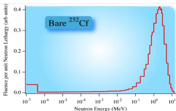
Figure 1: Energy spectrum of a  $^{252}\text{Cf}$  neutron source.
