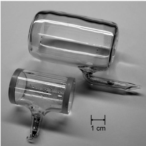
Figure 1: The smaller  $^3\text{He}$  cell was used as a sample inside the interferometer. The larger cell was used in polarization analysis. (Photograph by: NI&D group.)
