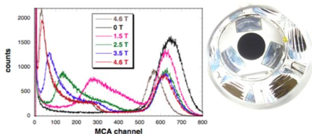
***On the top is shown the first version of the X-ray detector, in which the magnetic field was perpendicular to the APD electric field. These effect of the field on the response of the APD to 6 keV X-rays are shown in the bottom left plot. On the bottom right is shown the three-APD detector used for the radiative decay experiment, looking through the scintillator detector. (Photograph by: NI&D group.)***
