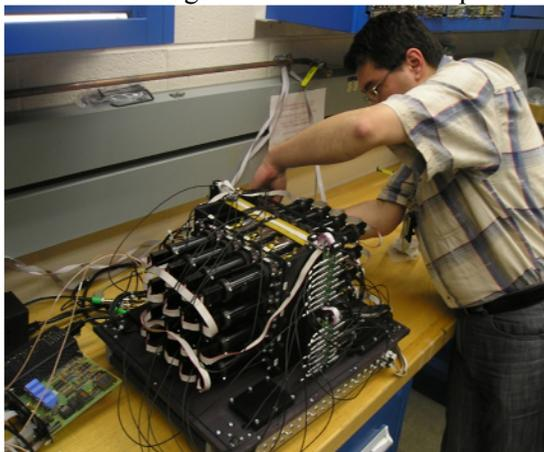
*Figure 1: Final assembly of the 16-channel neutron spectrometer. The detector was recently assembled and tested in the CNIF. (Photograph by: NI&D group.)*
