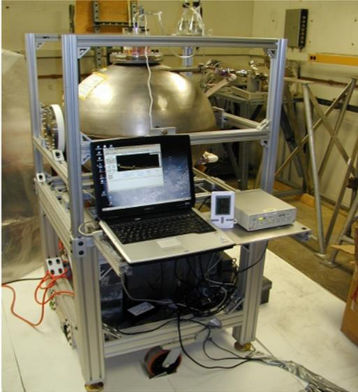
*A new reduced-volume manganese bath permits calibration of low-intensity neutron sources as required for DIIS applications. (Photograph by: NI&D group.)*
