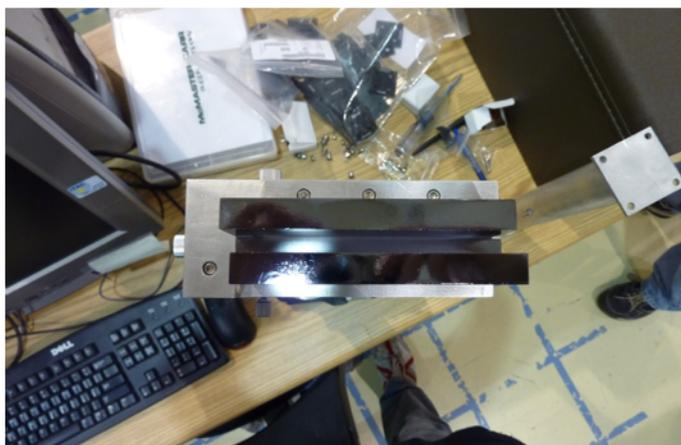
*Figure 2: Four vertical coils provide a smooth magnetic field around the crystal region. (Photograph by: NI&D group.)*
