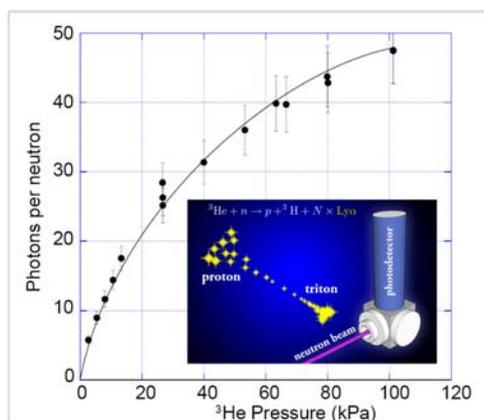
Figure 1: Lyman alpha photon yield per reacted neutron as a function of  $^3\text{He}$  pressure. The inset states the nuclear reaction and the cartoon indicates photon production and the experimental setup.
