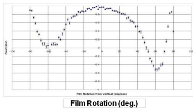
Figure 2: Polarization vs. single 10 micron permalloy film tilt.
