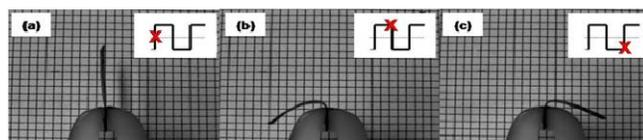
*Figure 1: IPMC actuation under applied electrical voltage. Each image was captured at the position of X on the excitation square wave*
