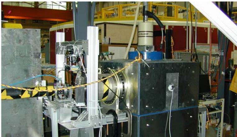
This is a new primary calibration method. It will be used to recalibrate the fluence monitor that was used in our beam-type neutron lifetime measurement, thereby simultaneously measuring the  ${}^6\text{Li}(n,t)$  and  ${}^{10}\text{B}(n,\alpha)$  thermal neutron cross sections, and to recalibrate the USA national neutron standard NBS-I.
