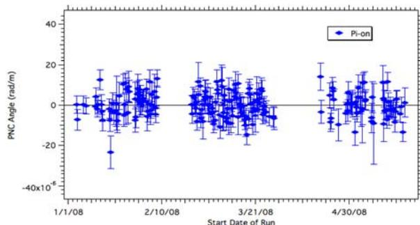
**Figure 2:** Results of the pi-coil on runs for the neutron spin rotation experiment. The rotation angle from each run is plotted as function of the time of the run throughout the entire experiment. The result of this experiment produced the best limit on the parity-nonconserving neutron spin rotation in liquid helium.
