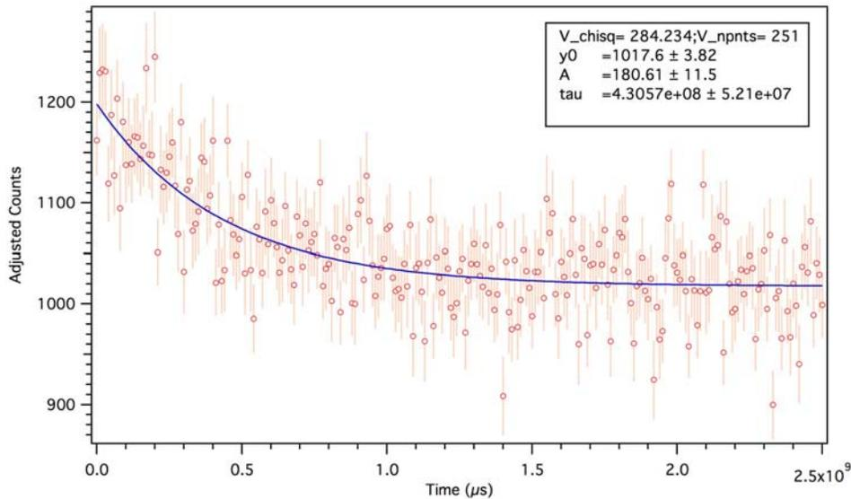
*Data from initial test runs at 50 %, showing the decay curve associated with the trap lifetime*
