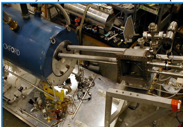
**Figure 1** Photograph of the apparatus on the NG-6 beam line. The neutron beam exits after traversing the LHe targets and the polarization is analyzed in with the supermirror and  $^3\text{He}$  ion chamber. (Photograph by: NIS&D group.)
