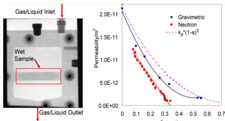
Figure 1: Left is a neutron image of the liquid and gas permeability measurement device. Right shows a comparison of the air permeability as measured by neutron radiography and gravimetrically, as well as a common functional form for the permeability as a function of saturation.
