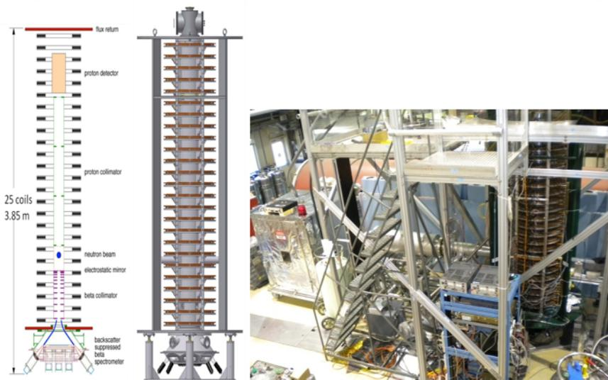
Two schematic diagrams of the apparatus is show on the left. The apparatus installed at our NG-6 beam position. (Photograph by: NI&D group.)
