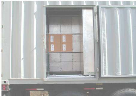
*An ISO Standard Cargo Container has been outfitted with the four cargo regions specified in N42.41. The section filled with hollow steel cubes can be seen. Part of each cargo region is on tracks to permit access to the central rack for threat specimens or stimulants. (Photograph by: NI&D group.)*
