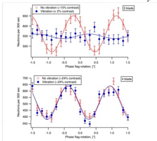
Figure 2: The fringe visibility for the MZ (top) and DF (bottom) type geometries. The DF type is insensitive to vibrations while the MZ is clearly not.
