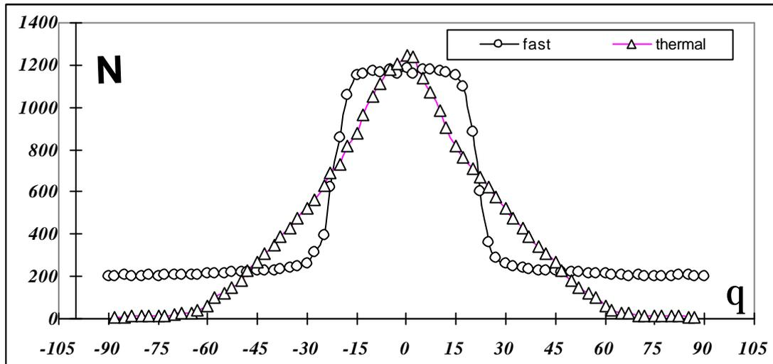
Thermal neutron fields were investigated with usage of indium and gold activation detectors, for investigation of fast neutron fields a radiometer of a type of a long-counter was applied.
