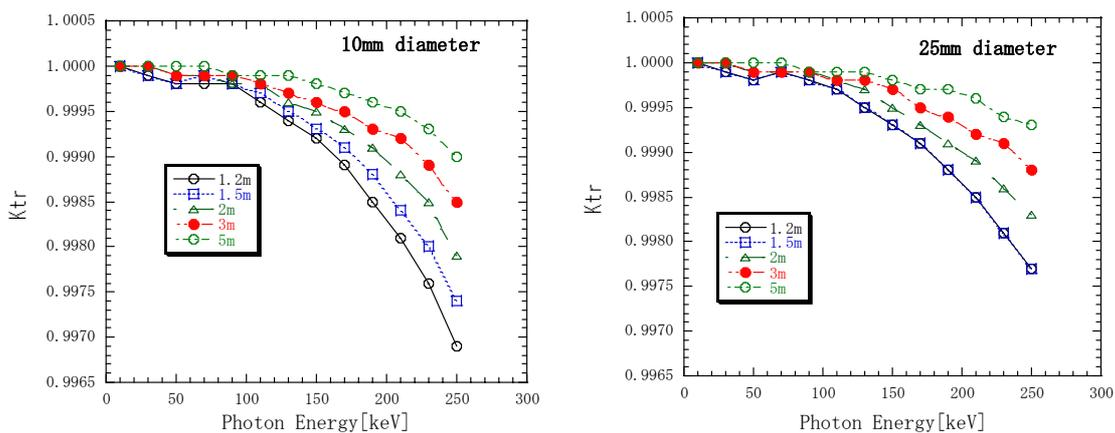
Figure 2. Correction factor  $K_{tr}$  for X-rays transmitted through the diaphragm edge for medium-energy free-air chamber. Left: 10-mm diameter aperture, right: 25-mm diameter aperture.
