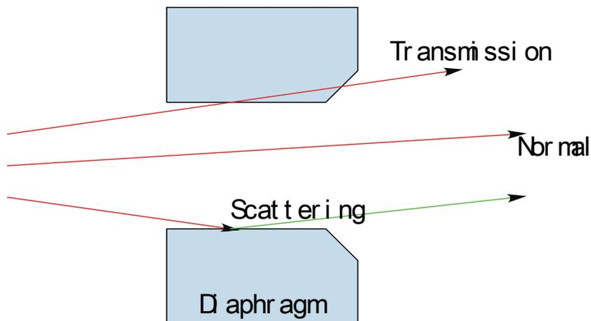
Figure 1. Schematic view of X-rays entering into a free-air ionization chamber through the diaphragm.
