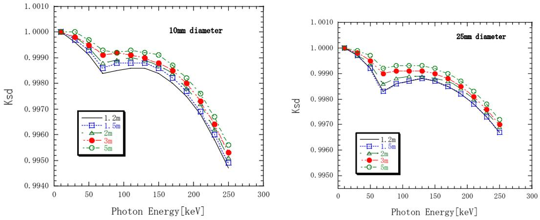
Figure 3. Correction factor  $K_{sd}$  for X-rays scattered at the surface of the diaphragm aperture for medium-energy free-air chamber. Left: 10-mm diameter aperture, right: 25-mm diameter aperture.
