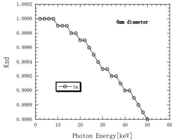
Figure 4. Correction factor  $K_{sd}$  for X-rays scattered at the surface of the diaphragm aperture for low-energy free-air chamber.
