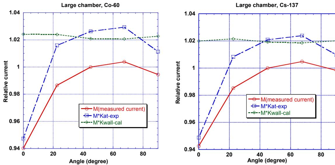
Figure 3. Changes in the measured currents. Those currents corrected for attenuation obtained by experimental methods and those currents corrected for wall effects obtained by calculation. All values are normalized using currents measured at 45 °.
