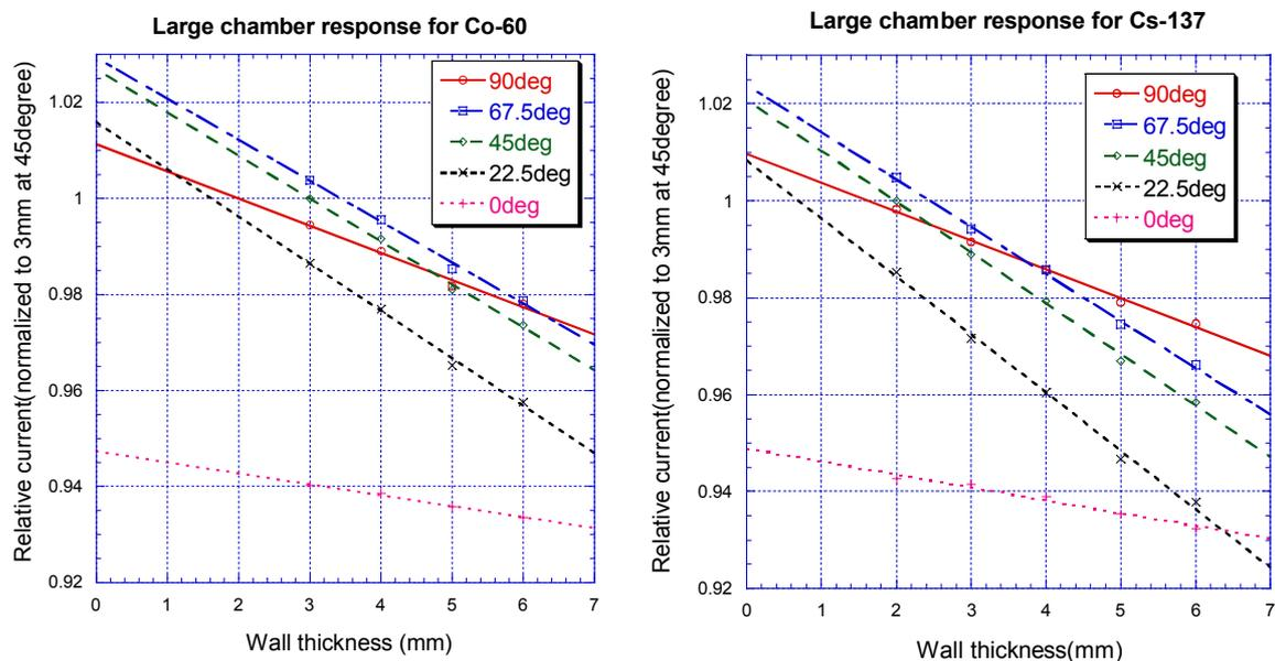
Figure 2. Relative signal currents from the ionization chamber plotted as a function of incident wall thickness for various angles of gamma rays.
