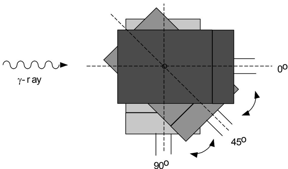
Figure 1. Setup of the cavity chamber in gamma ray fields. Incident angles of the gamma rays on the chamber are shown. The chamber is turned on a horizontal plane around the vertical axis around the center of the ionization volume of the chamber.
