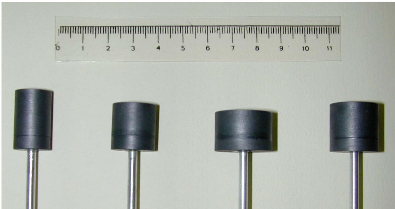
**Figure 1** – Photo of the four ionization chambers (from the left, chamber code A, B, C, D) of various shape and size built for the present study.
