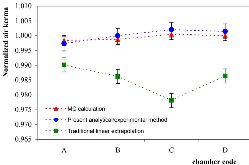
**Figure 2.** Air kerma values determined by the different ion chambers (A, B, C and D) using  $K_{wall}$  factors obtained by the three methods specified in the graph (triangles, circles and squares). The data are normalized to the MC value of the chamber D.
