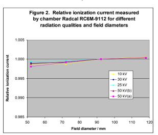
The field sizes in use in laboratories holding free-air chambers for low-energy x-rays range from 60 mm to 100 mm, the value at the BIPM being around 85 mm. Over this range of field
