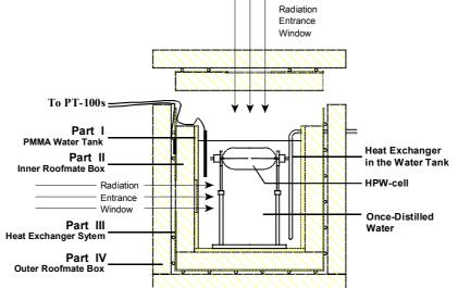
comprising of two AC-Wheatstone bridges in combination with two lock-in amplifiers. The calorimeter has extensively been tested in the <sup>60</sup>Co gamma
