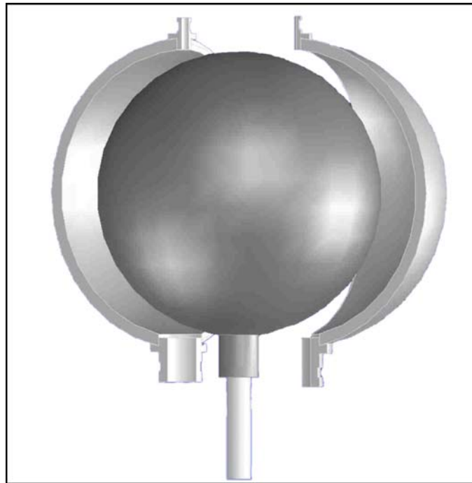
Figure: Sketch of the optimized secondary standard chamber for H^*(10)
