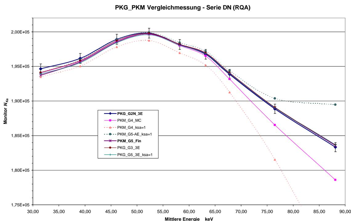
Figure 1 PKM aperture optimization process with final comparison PKM/PKG (PKM\_G5 Final aperture design was compared with PKG\_G2N\_3E and PKG\_G3\_3E measurements)
