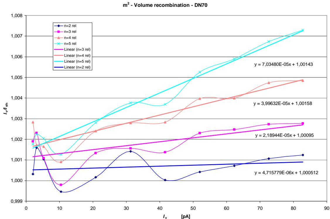
Figure 2. Ratio of the ionization currents  $I_V$  and  $I_V/n$  measured in PKM chamber with voltages  $V$  and  $V/n$  respectively, as a function of  $I_V$ , for several  $n$  values
