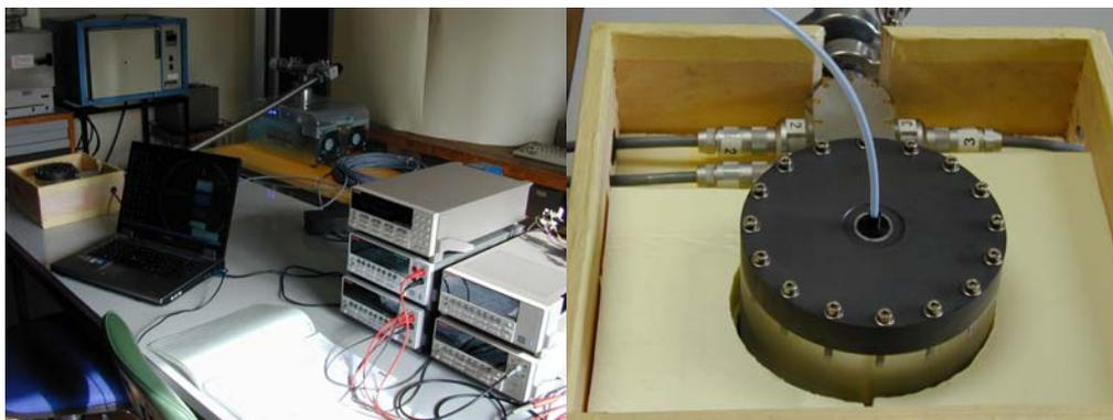
**Figure 3.** The electronic equipment for controlling the calorimeter is composed of a switching frame Keithley 7001, 2 precision power supply Keithley 2400. A fast current source Keithley 6220 coupled to a DC nanovoltmeter Keithley 2182A is used for resistance variation measurements (left). The catheter that drives the  $^{192}\text{Ir}$  source is inserted in the calorimeter (right).
