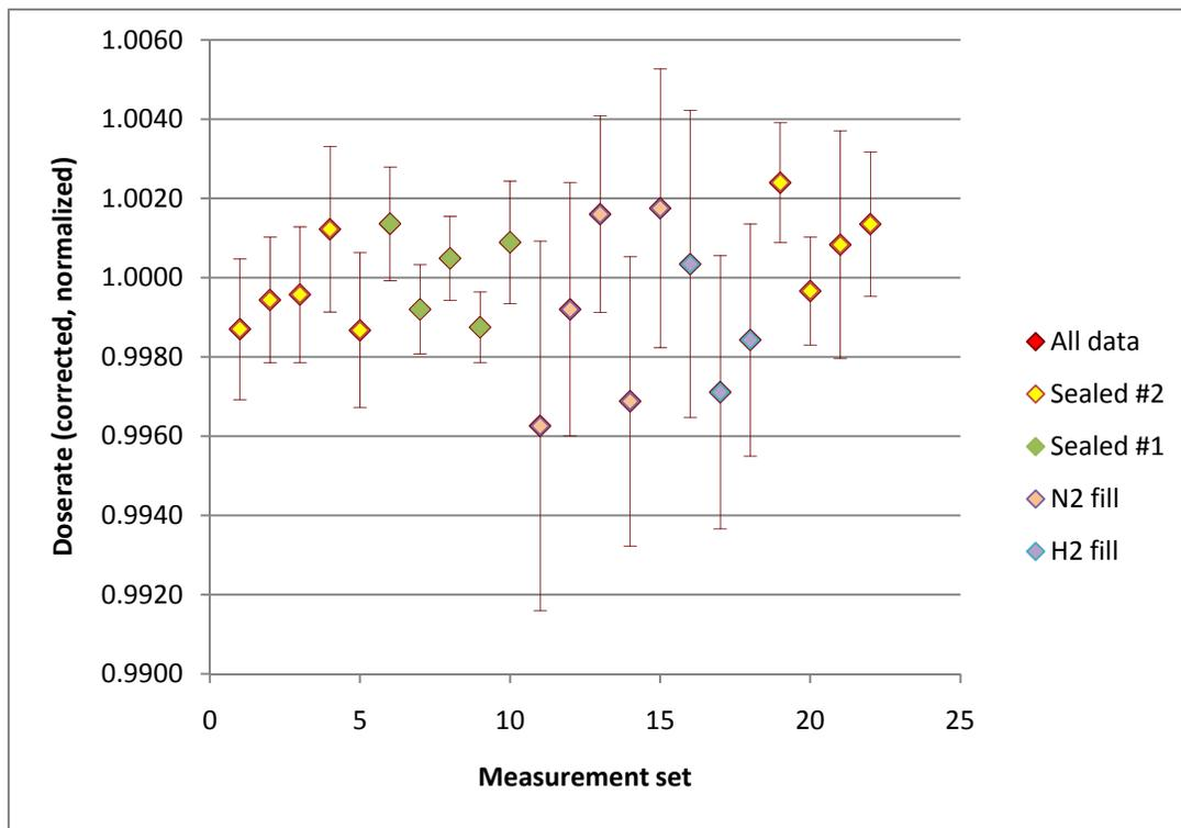
**Figure 1.** Water calorimetry measurements on the NRC <sup>60</sup>Co beam. Each set represents typically 15 individual runs. The absorbed dose rate to water was determined to be 2.542 cGy sec<sup>-1</sup>.
