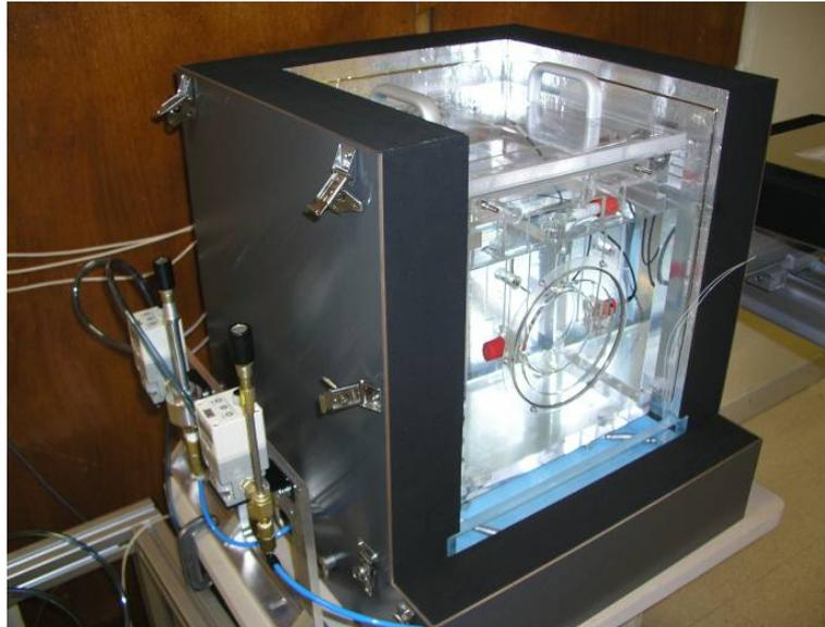
*Water calorimeter for small depth measurements*
