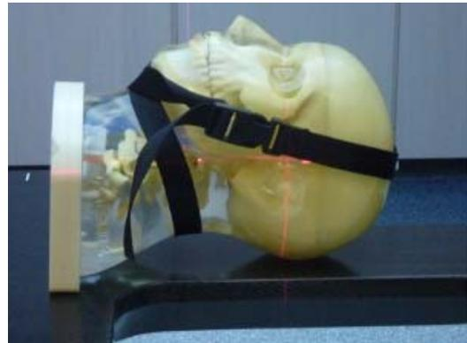
*PMMA cylinder and anthropomorphic head*
