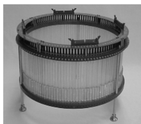
Photograph of the transducer array for ultrasound tomography. (Photograph used with permission from Luna Innovations, LLC.)
