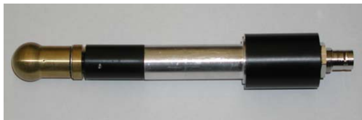
The NIST prototype cavity chamber used to determine air-kerma rates. (Photograph by: Ronaldo Minniti)
