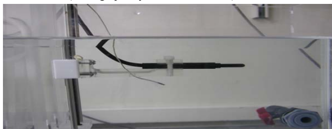
Setup of absorbed dose to water measurement. (Photograph by: Ronaldo Minniti.)
