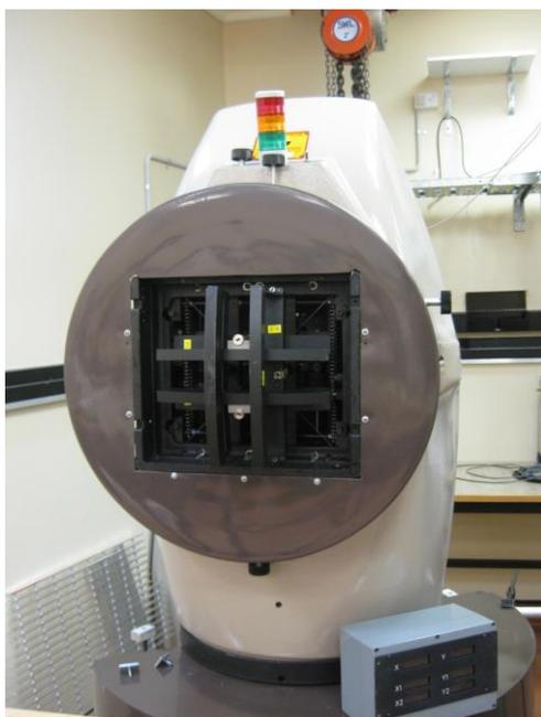
**Figure 1.** Eldorado 78  $^{60}\text{Co}$  therapy treatment head installed in 2009
