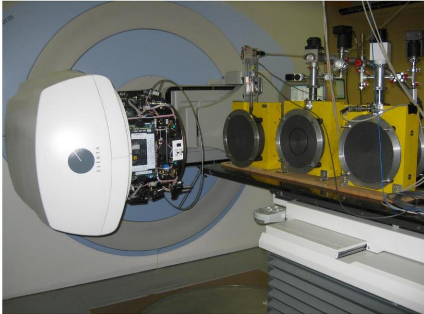
**Figure 2.** The ARPANSA and IAEA calorimeters on the patient support table at the measurement distance from the therapy head. The third device on the table at far left is a graphite phantom holding a thimble chamber.
