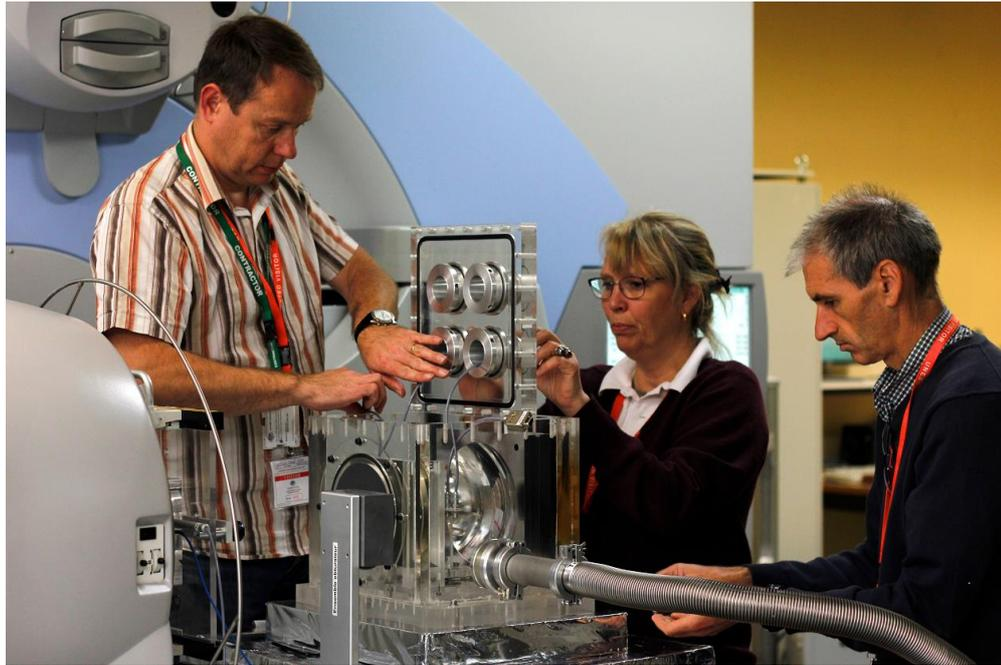
**Figure 3:** BIPM staff Philippe Roger (left), Susanne Piccard and David Burns installing the BIPM calorimeter on the Elekta Synergy Linac at ARPANSA.
