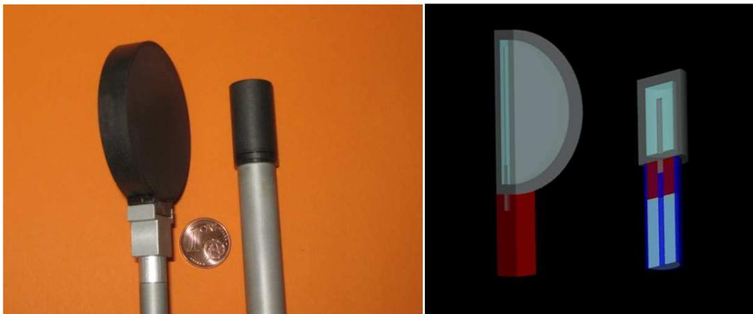
Figure 1.3: The cavity ionization chambers used for the benchmark measurement (left) and the models of the chambers used for the Monte-Carlo calculations (right).
