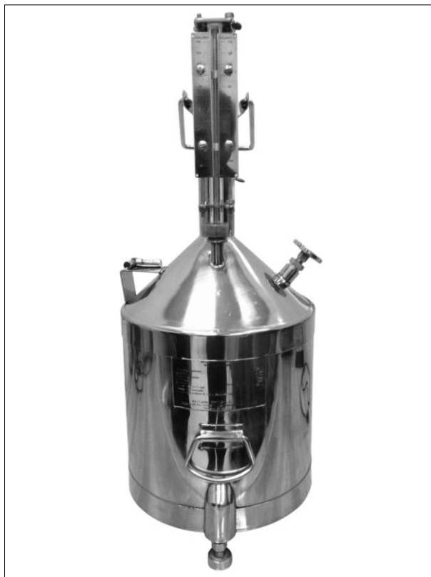
Fig. 2. Image of the 20 L graduated neck test measure. TS 04.
