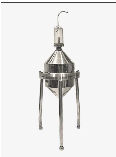
Fig. 1. Image of the overflow type 20 L pipette. TS 710-05.
