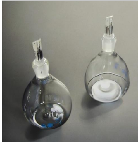
Fig. 3. Image of the TS for 100 mL. Glass pycnometers 03.01.15 and 03.01.17.
