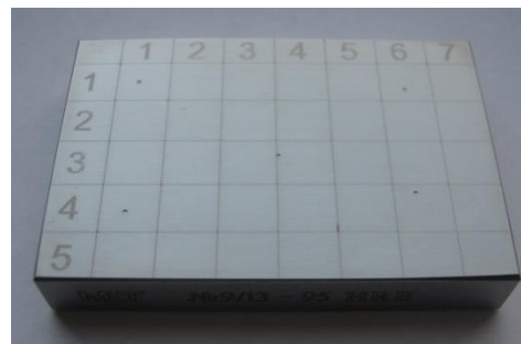
Figure 3 Layout of the grid on the measurement surface of the hardness reference blocks
