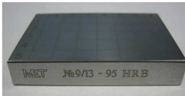
Figure 2 Hardness reference blocks used for the HRB RKC with the logo of the manufacturer
