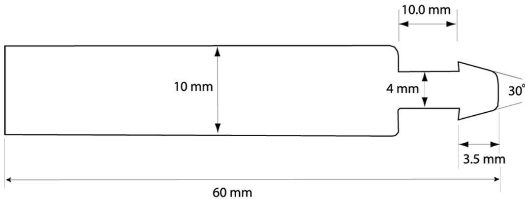
**Figure 4.** The striker cross section provides approximate dimensions for the instrumented striker used in this comparison. The strain gauges are positioned on both sides of the 4 mm-thick beam that supports the striking edge. The center of the gauge is approximately 7 mm behind the leading edge of the striker and 12 mm below the top of the striker. The center of strike is about 10 mm from the top of the striker. The radius of the striking edge is 8 mm, in accordance with ASTM E23-18 [6].
