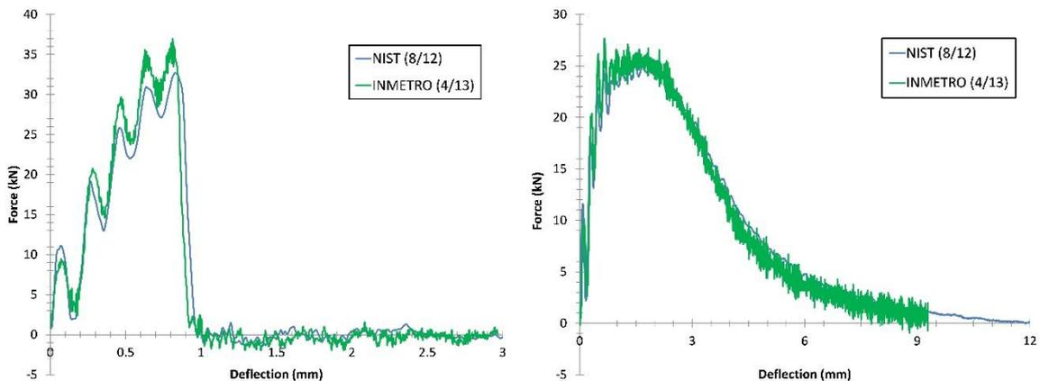
**Figure 1.** Comparison of representative instrumented curves for low-energy specimens (left) and high-energy specimens (right) from the 1<sup>st</sup> and 3<sup>rd</sup> test series.
