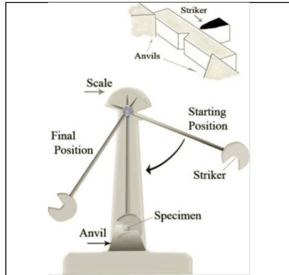
**Figure 2 - In a Charpy test, a pendulum (of known mass and length) is released from a starting height and impacts a specimen positioned against two anvils.**
