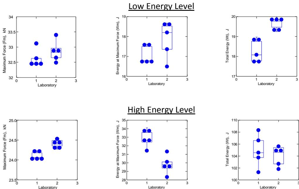
**Figure 6.** Box plots comparing results for laboratories 1 and 2 for  $F_m$ ,  $W_m$ , and  $W_t$  for the low- and high-energy levels.
