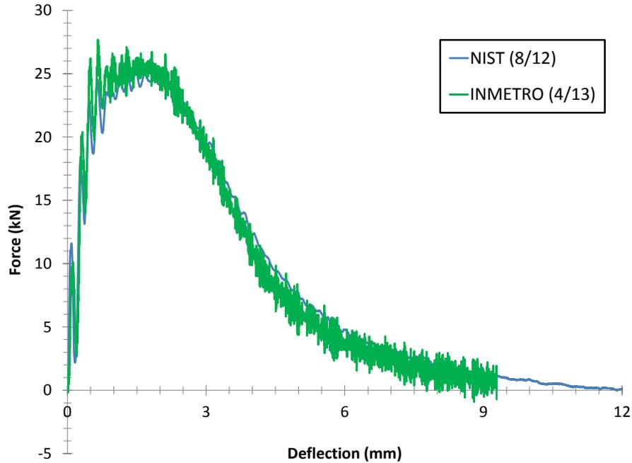
**Figure 8.** Comparison of representative curves for high-energy specimens from the 1<sup>st</sup> and 3<sup>rd</sup> series.
