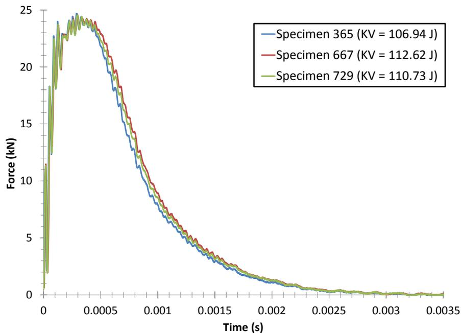
**Figure 5.** Comparison between instrumented force/time traces for three high-energy specimens from the 1<sup>st</sup> test series (Lab 01).
