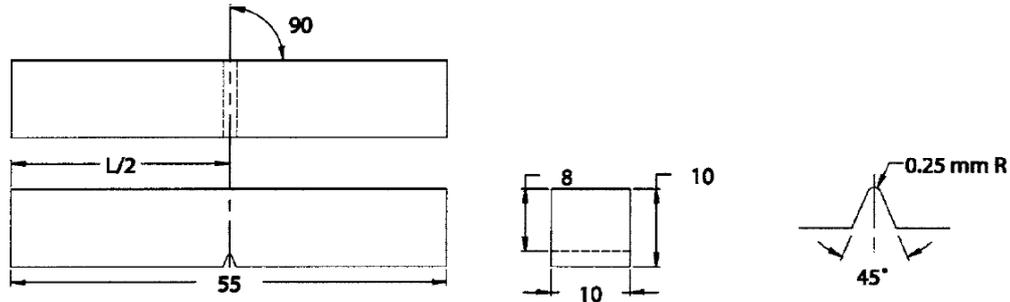
**Figure 3.** Dimensions of the Charpy V-notch verification specimen (millimeters).
