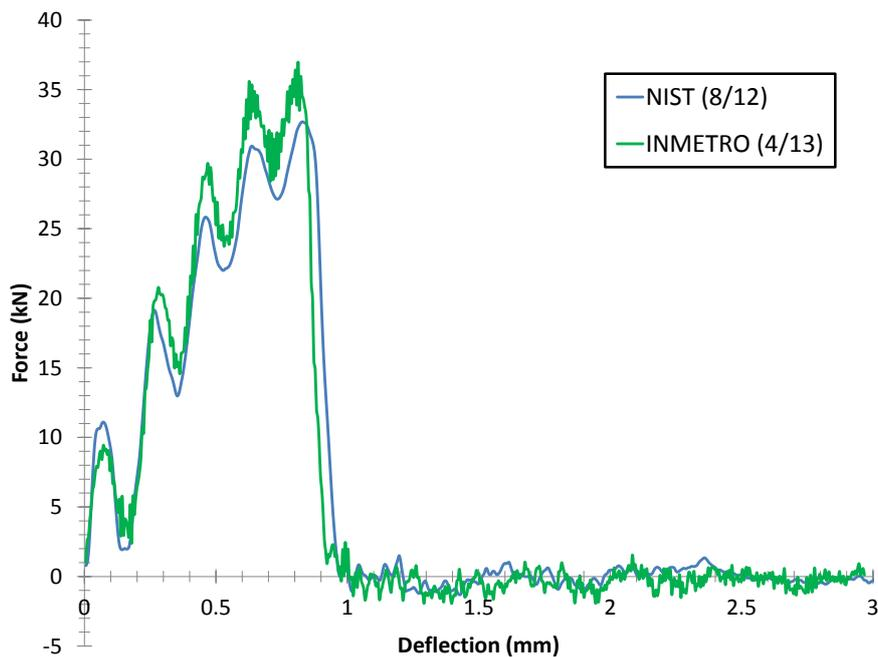
**Figure 7.** Comparison of representative curves for low-energy specimens from the 1<sup>st</sup> and 3<sup>rd</sup> series.
