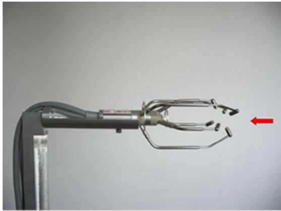
**Figure 3 - Ultrasonic Anemometer sensing element; the arrow indicates the flow direction**
