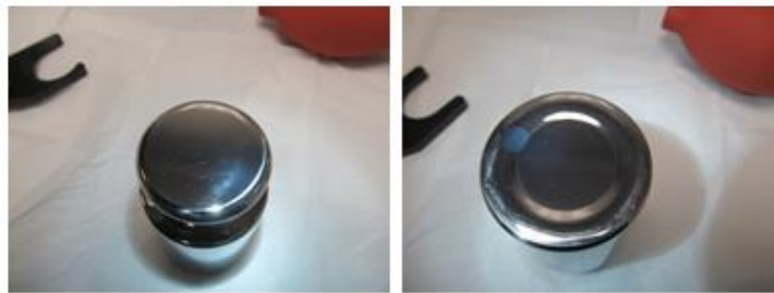
Image 2. Scratches on the surface of 1 kg weight after circulation
