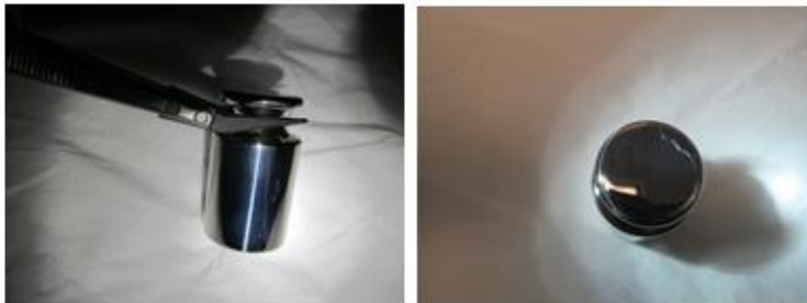
Image 3. Scratches on the surface of 200 g weight after circulation
