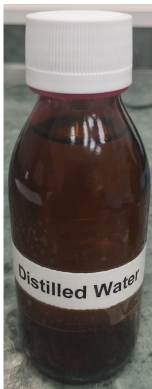
Figure 2 Distilled Water Liquid sample for the comparison in a glass bottle with a nominal volume of 80 cm 3
