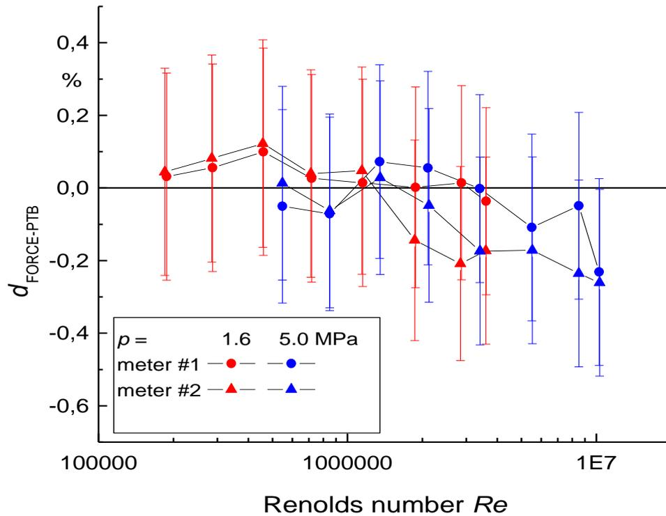
Fig. 4.3: Plot of bilateral differences NIST-PTB versus Reynolds number  $Re$  both meters;
