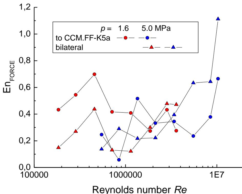
Fig. 5.1: Plot of degree of equivalence ( $En$ ) versus Reynolds number  $Re$  (average of both meters);
