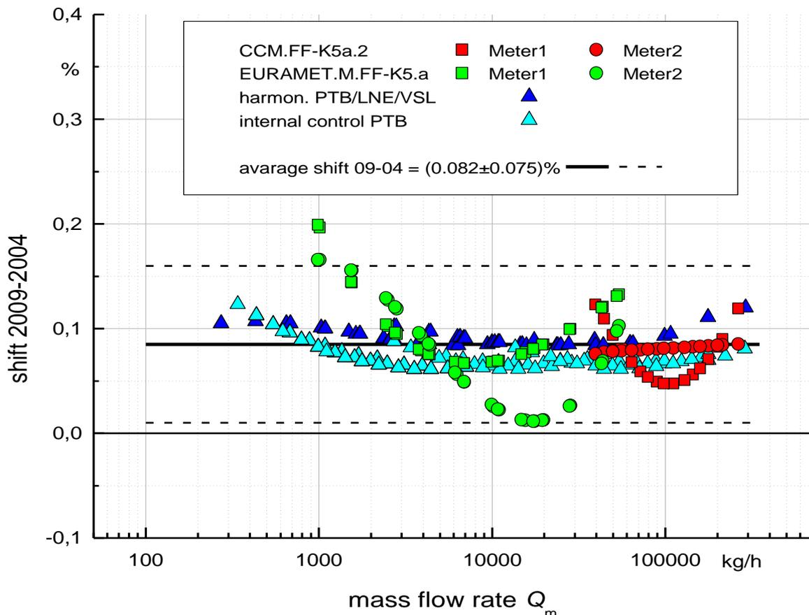
Fig. 3.2: Shift in the calibration values for meters under test at PTB-pigsar due to recalibration 2007 for different sets of meters.
