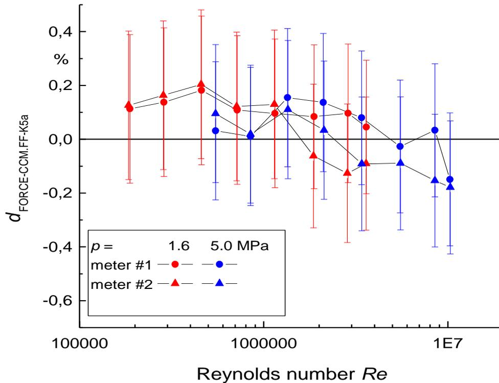
Fig. 4.4: Plot of differences  $FORCE-KCRV_{CCM.FF-K5a}$  versus Reynolds number  $Re$  both meters (turbine and USM);
