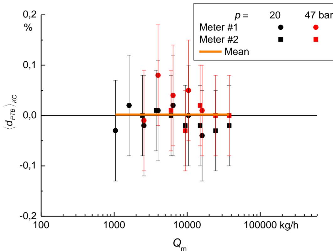
Fig. 3.3: Results for the difference of PTB  $\langle d_{PTB} \rangle_{KC}$  to the KCRV in the CCM.FF-K5a.
