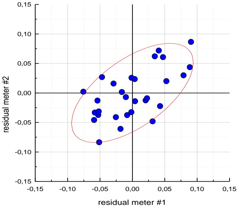
Fig. 3.1: The correlation plot of two meters within EURAMET.M.FF-K5a determined at the pilot laboratory using the difference (residuals) between the single measurement results  $f_{meter\#i}$  and the average value  $f_{ave\#i}$  (least square fit of test result measured at 1600 kPa and 5000 kPa in March and September 2009).
