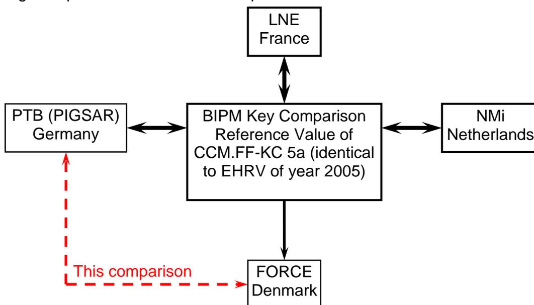
Fig. 1: The traceability of the participants in relation to the BIPM Reference Value of CCM.FF-KC5a and the position of this bilateral inter comparison
