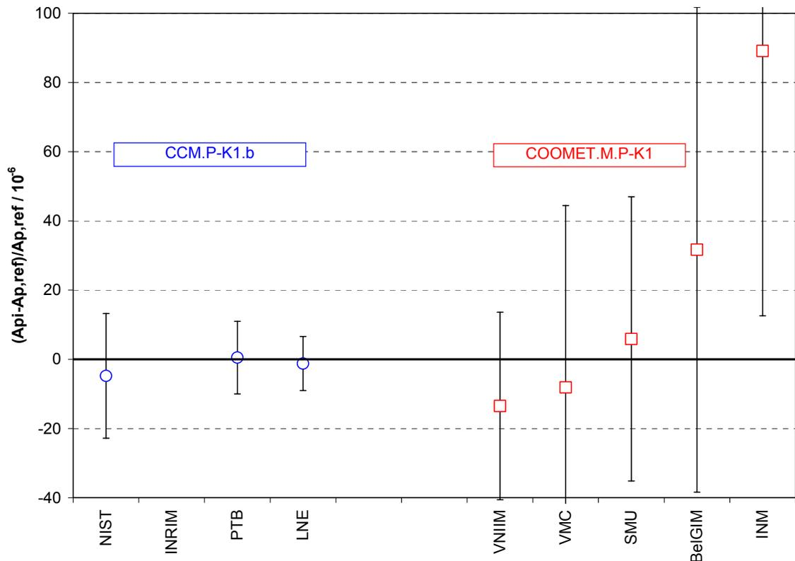
**Figure 3.1** Relative deviations of the participants results' from the reference value of comparison CCM.P-K1.b and the expanded ( $k=2$ ) uncertainties of these deviations at 50 kPa
