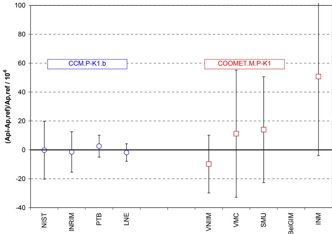
**Figure 3.4** Relative deviations of the participants results' from the reference value of comparison CCM.P-K1.b and the expanded ( $k=2$ ) uncertainties of these deviations at 400 kPa
