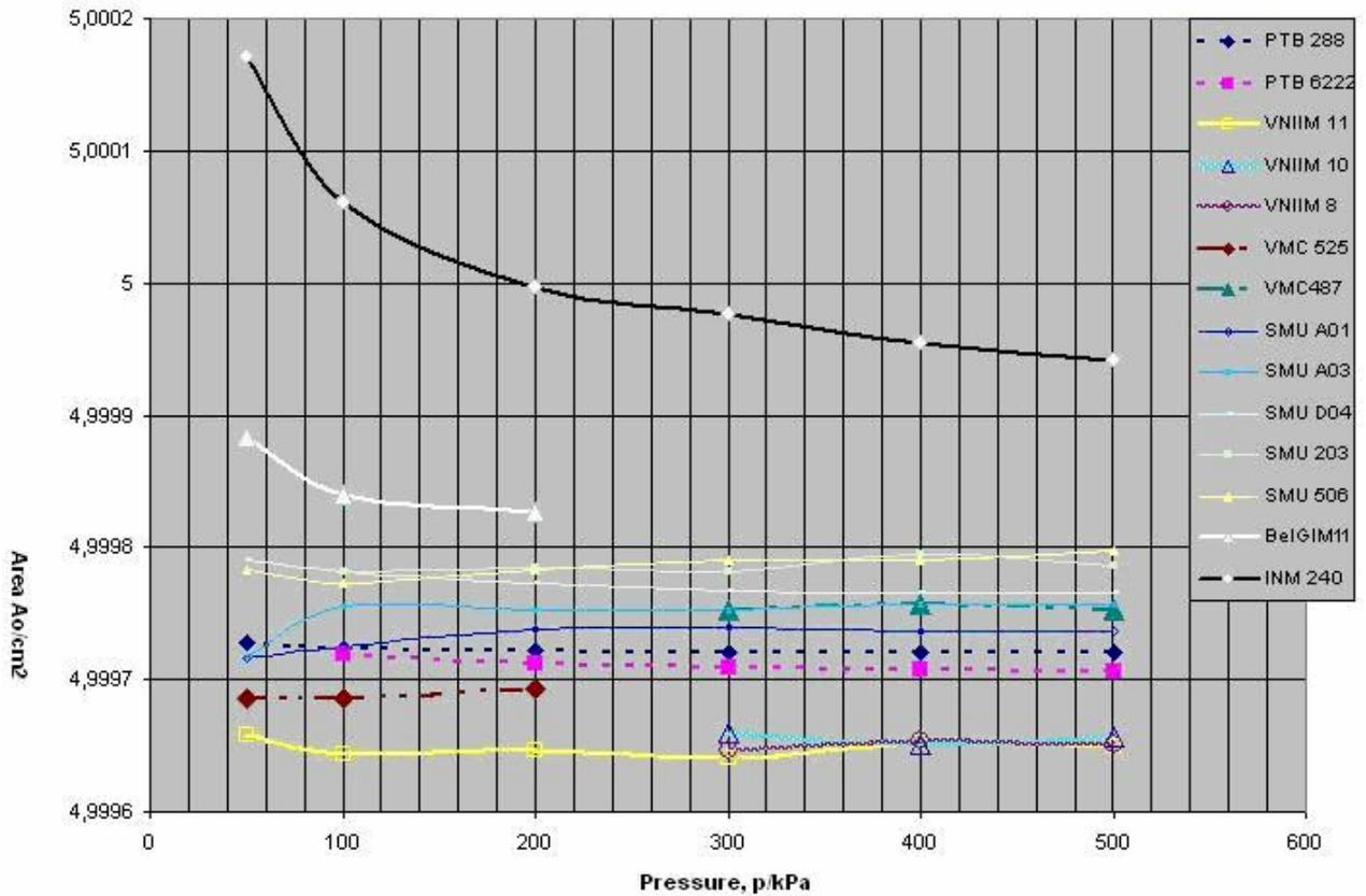
**Figure 1** Effective area of the TS determined from comparison with the NPS of VNIIM, PTB, VMC, SMU, BelGIM and INM.
