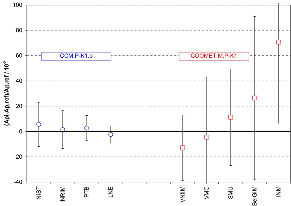
**Figure 3.2** Relative deviations of the participants results' from the reference value of comparison CCM.P-K1.b and the expanded ( $k=2$ ) uncertainties of these deviations at 100 kPa
