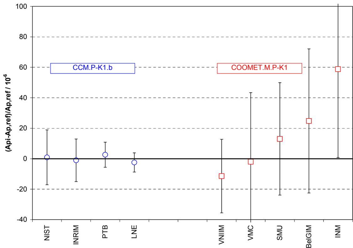
**Figure 3.3** Relative deviations of the participants results' from the reference value of comparison CCM.P-K1.b and the expanded ( $k=2$ ) uncertainties of these deviations at 200 kPa
