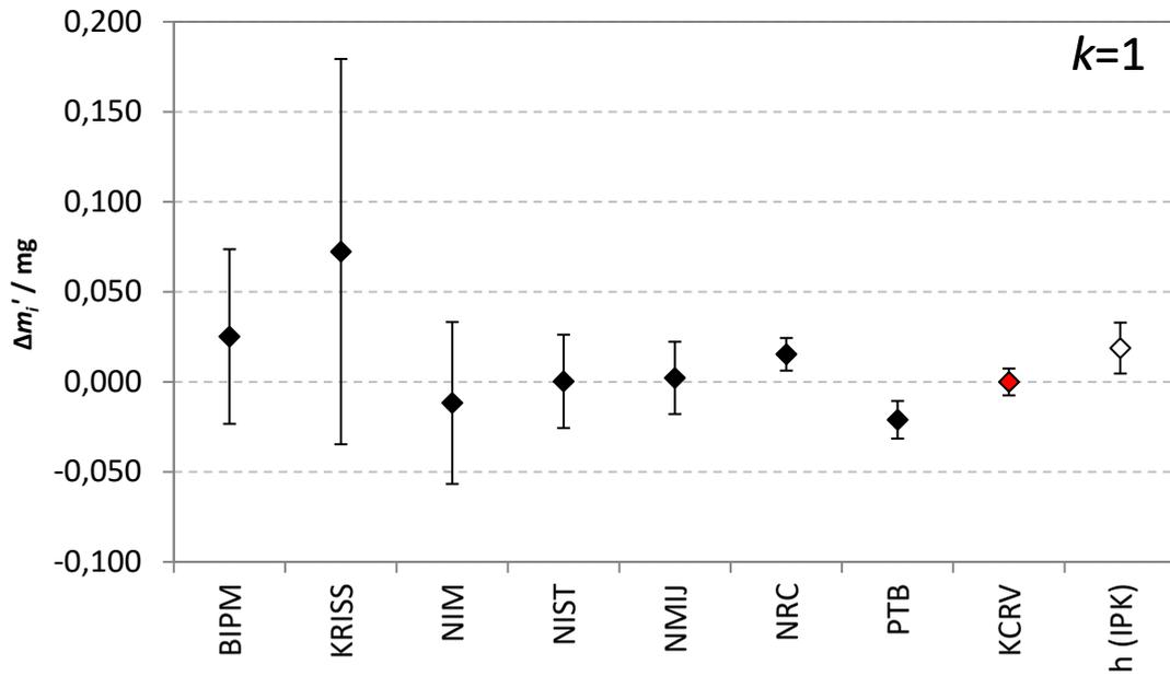
**Fig. 3:** Differences  $\Delta m_i$  between mass values attributed to 1 kg mass standards using the realization experiment of the participants and the KCRV, calculated as the weighted mean. The difference between the realization based on the BIPM working standards, traceable to the Planck constant through the IPK, and the reference value is also indicated.
