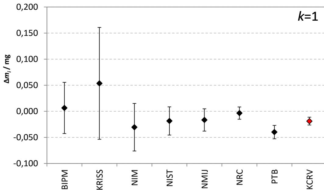
**Fig. 2:** Differences  $\Delta m_i$  between mass values attributed to 1 kg mass standards using the realization experiment of the participants and by the working standards of the BIPM, and associated standard uncertainty.
