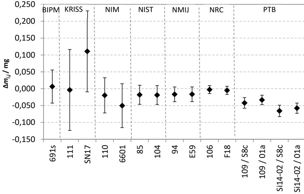
**Fig. 1:** Differences  $\Delta m_{i,j} = m_{i,j}^{\text{NMI}} - m_{i,j}^{\text{BIPM}}$  between the mass determinations of each travelling standard with the NMI's realization experiment and the BIPM working standards and associated combined standard uncertainties
