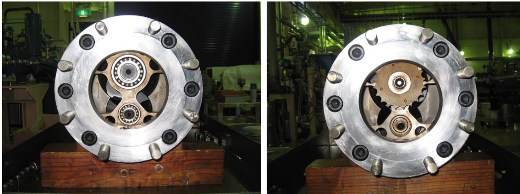
Fig. A1-7 Pictures of the inlet and outlet of the PD meter.
