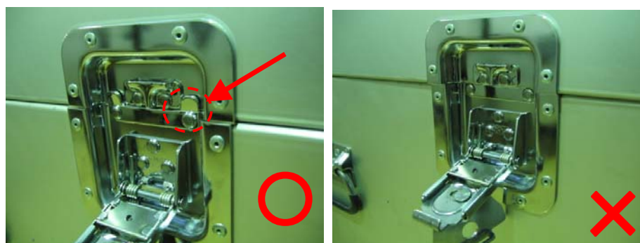
Fig. A1-5 Projecting guides of a rotary lock should appear when a box is closed.
