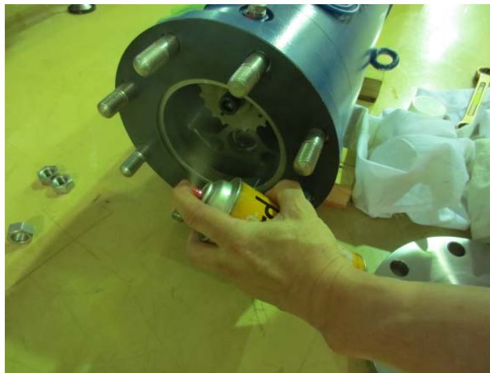
Fig. A1-10 Give the anti-rust treatment (ex. anti-rust spray) to the wetted part of the PD meter.
