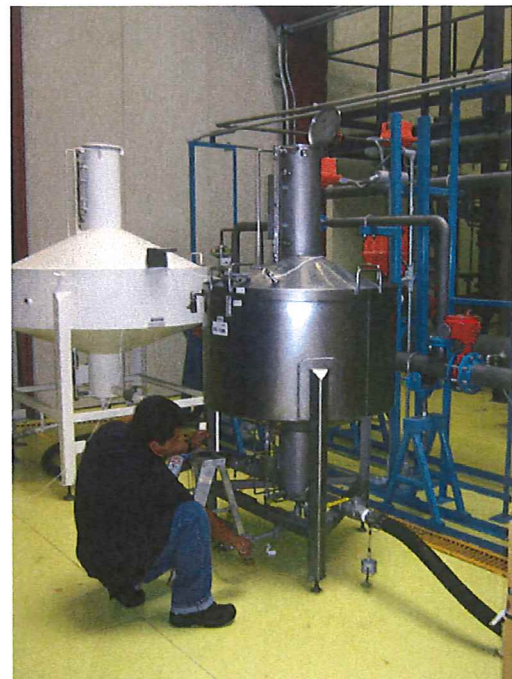
Fig. 8 General view of the water flow facility, CENAM was used a 500 L volumetric standard
