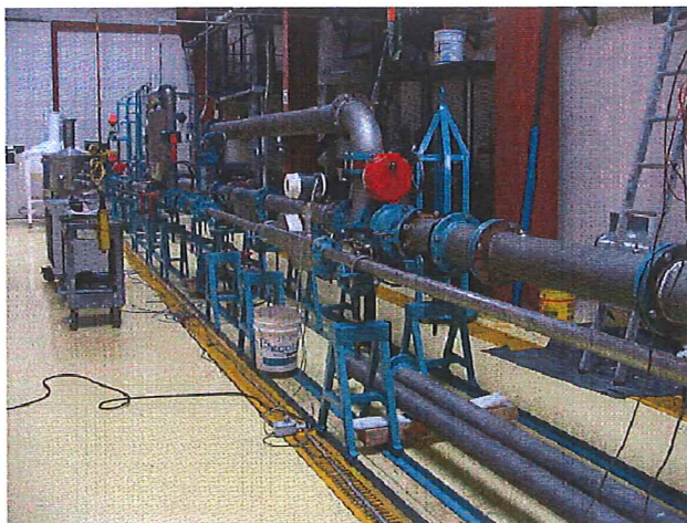
Fig. 8 General view of the water flow facility, CENAM was used a 500 L volumetric standard
