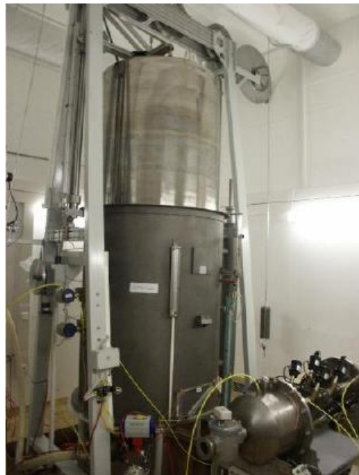
Fig. 5. Gas flow standards.
