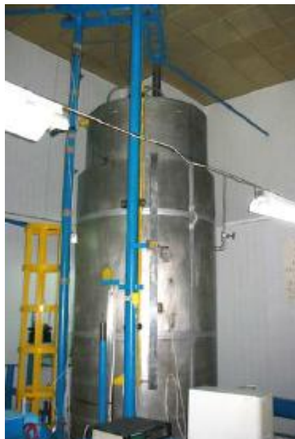
Fig. 3. The National gas flow standard ДЕТУ 03-01-96
