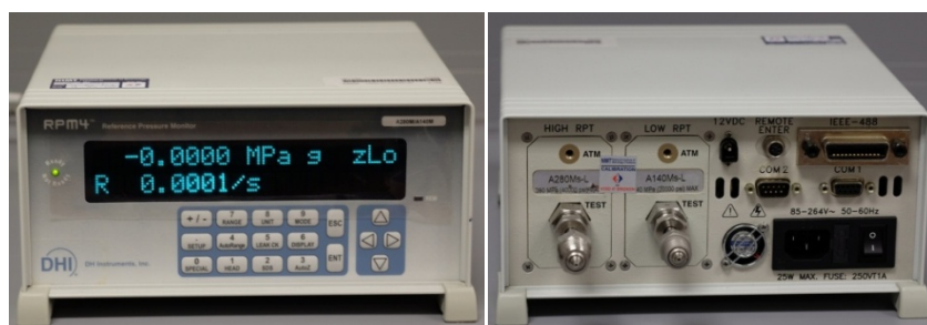
Figure 1. TS[1] hydraulic reference pressure monitor, Model: RPM4 A280M/A140M, S/N: 556.
