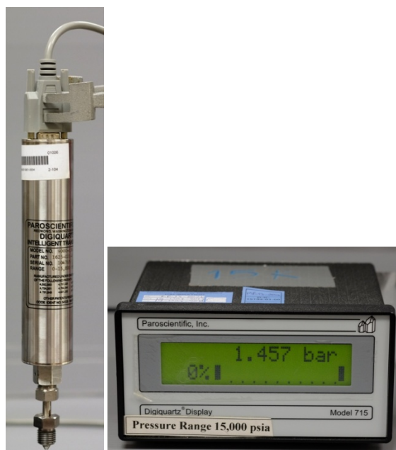
Figure 2. TS[2] hydraulic pressure transducer, Model: 9000-15K-101, S/N: 104765 and digital precision indicator, Model: 715-220V, S/N: 924.
