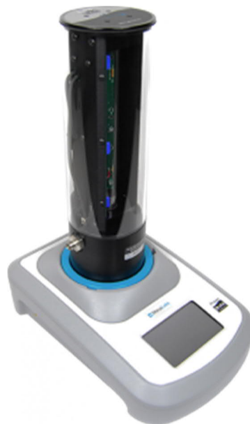
Figure 3. Mesa Labs DryCal 800 system including base and flow cell. A set of three flow cells were used to cover the flow range of the comparison.
