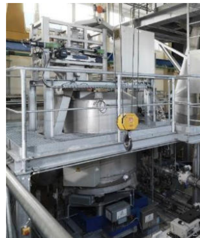
3 t balance and diverter system
