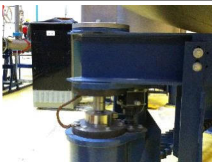
Fig. 2: A view of the load cell at the 10 000 kg tank
