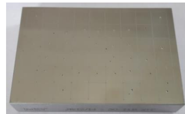
Figure 3 Layout of the grid on the measurement surface of the hardness reference blocks
