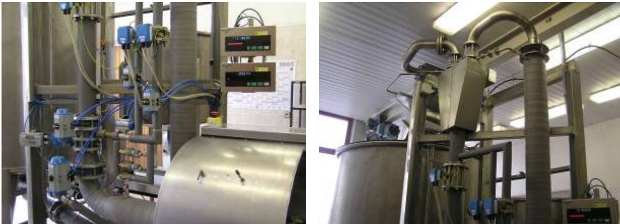
Fig.5.1 The water flow test rig of CMI
