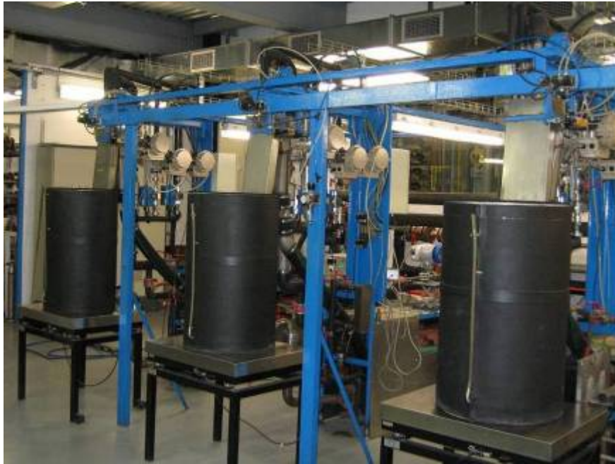
Fig.5.9 Part of the water flow calibration facility of CETIAT (France)
