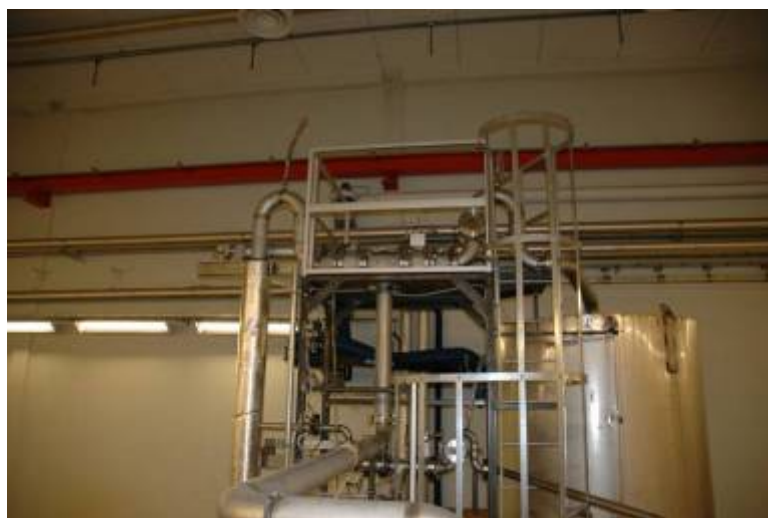
Fig.5.3 T-pipe section of the test flow rig at JV
