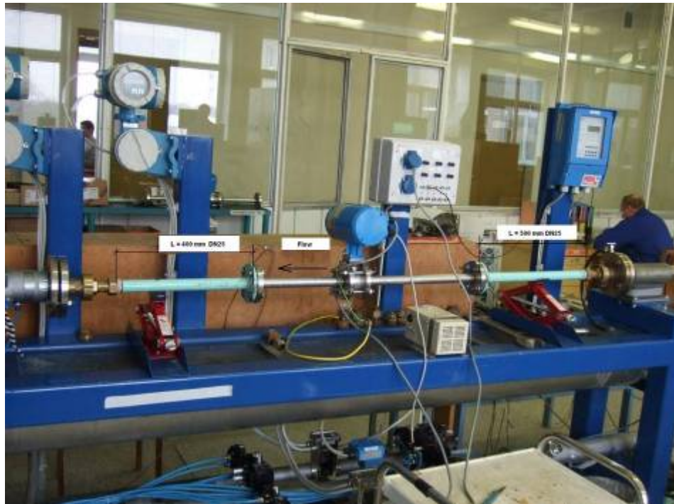
Fig.5.12 Installation of the meter in VMT/LEI
