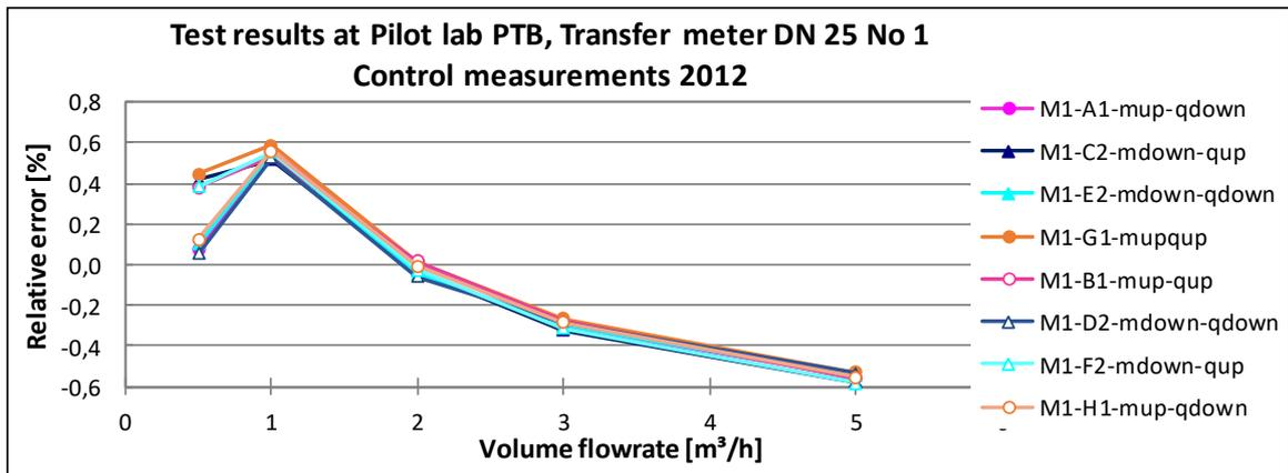
Fig. 8: Measurement error of transfer meter 1 (turbine meter DN25) - calibrated at PTB during the years of 2009, 2010 and 2012
