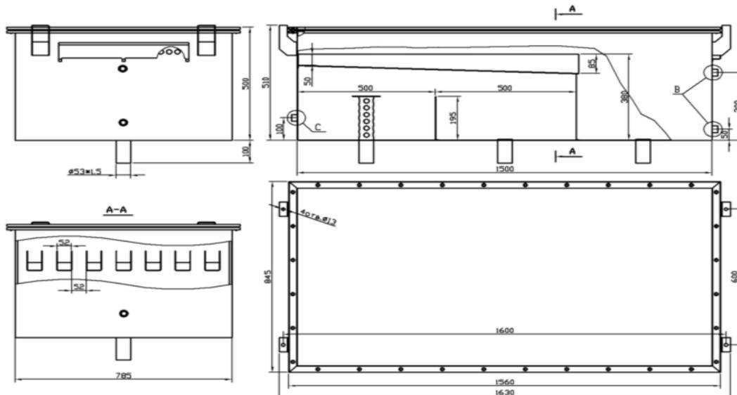
**Figure A.14** - Constant level head tank of the installation
