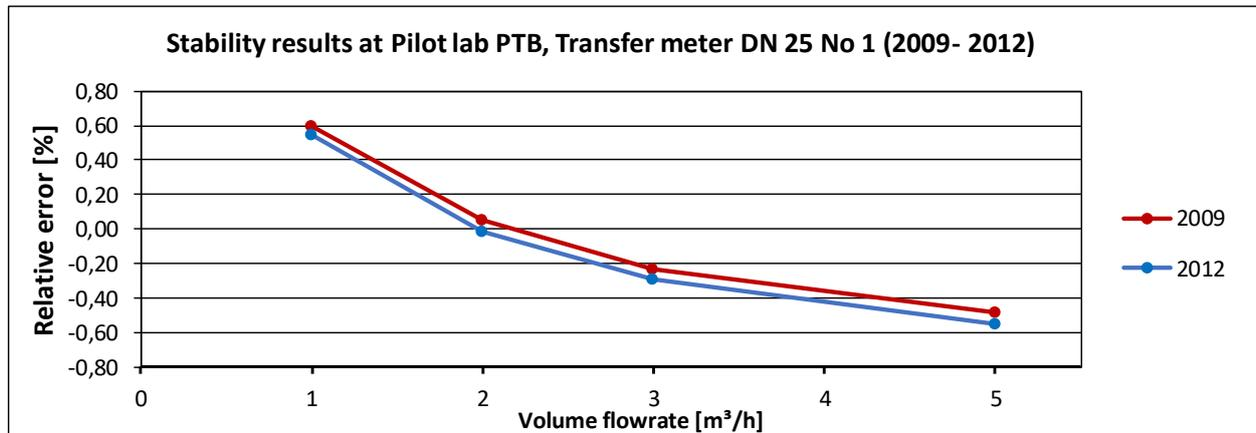
Fig. 10: Turbine flowmeter M1 - Stability during calibration period between 2009 and 2012 at pilot laboratory - The measurement errors are representing mean values, calculated by using all measured data of different calibration variations for each flowrate.
