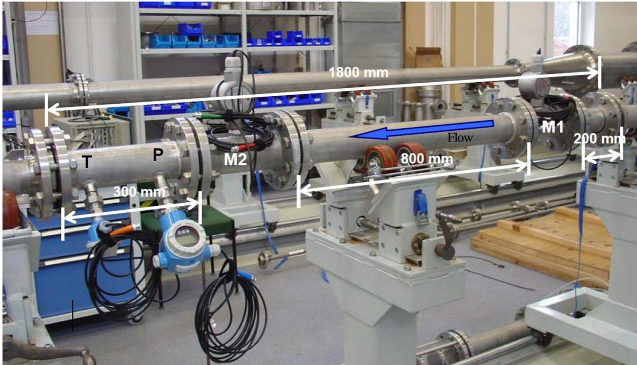
Fig. 14: DN80 transfer standards installed in calibration line at PTB
