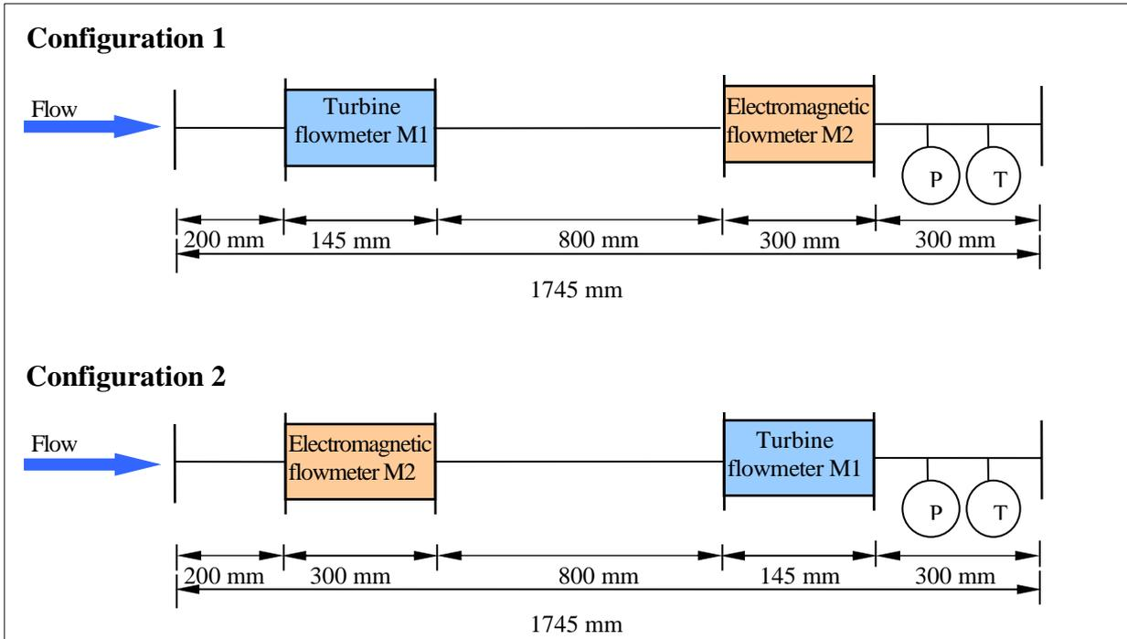
Fig. 6: Measurement configurations for the DN25 transfer standard
