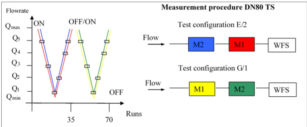
Fig. 5: Measurement procedure E2 and G1 for DN80 transfer standards
