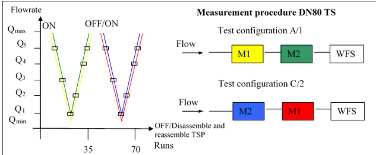
Fig. 4: Measurement procedure A1 and C2 for DN80 transfer standards
