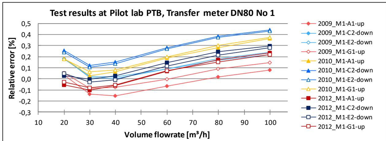
Fig. 15: Turbine flowmeter DN 80 M1 – Measurement error of the calibrations at PTB
