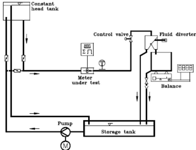
**Figure A.2.** Gravimetric part of the standard
