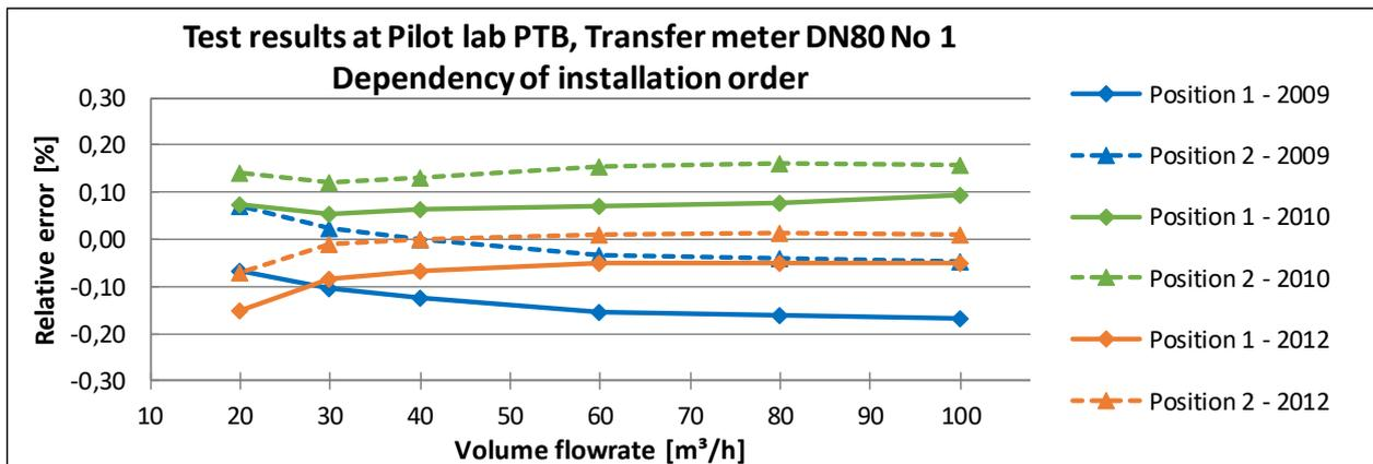
Fig. 17: Turbine flowmeter M1 – Deviation to mean of measurement errors in dependency of installation order (upstream - position 1, downstream - position 2) for comparable measurement conditions (e.g. day 1/4 to day 2/3, given as A1/G1 to C2/E2)
