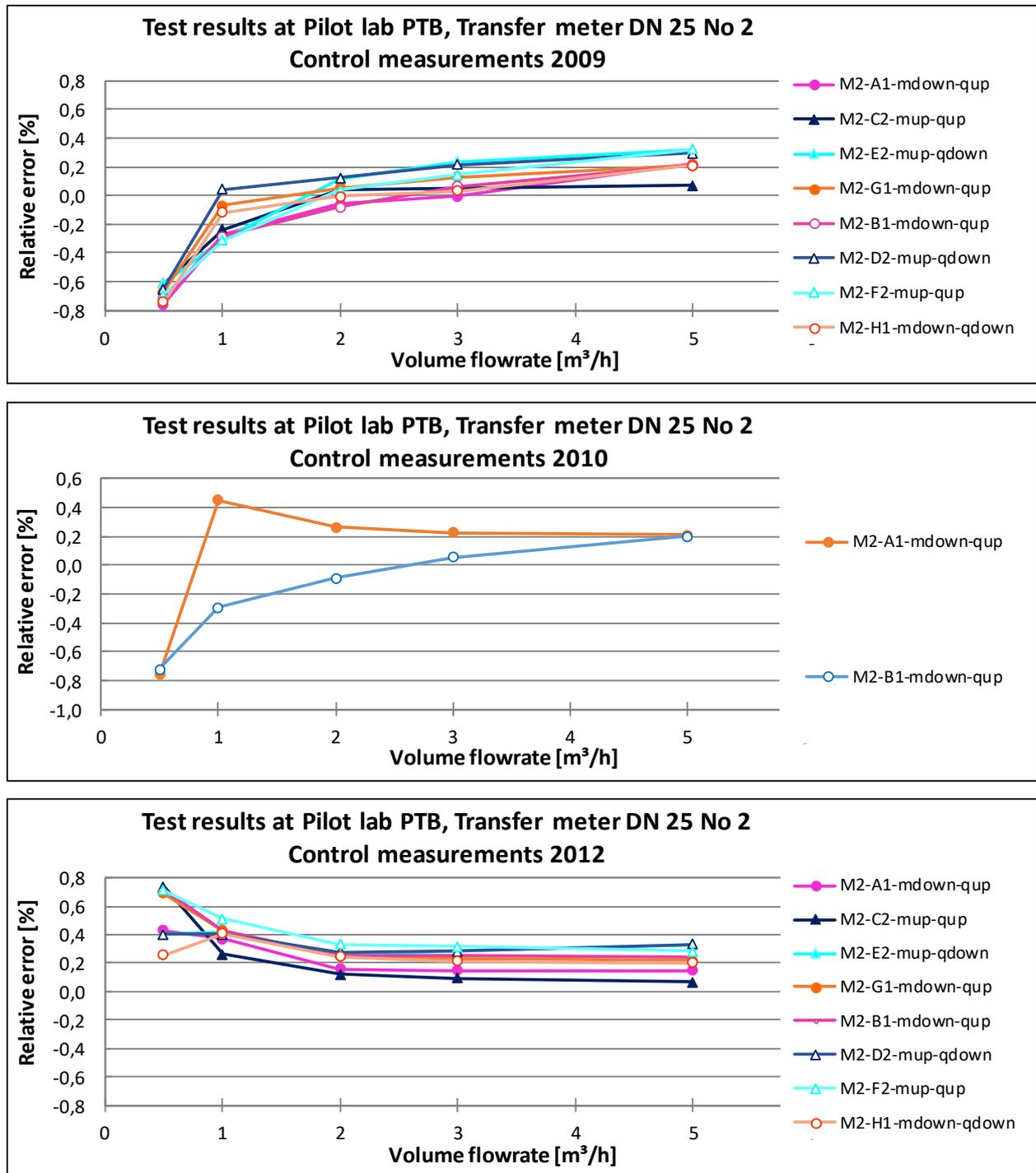
*Fig. 11: Electromagnetic flowmeter M2 DN 25 - Measurement errors of the calibrations at PTB with: M2 - Meter 2 (Electromagnetic flowmeter DN 25)
