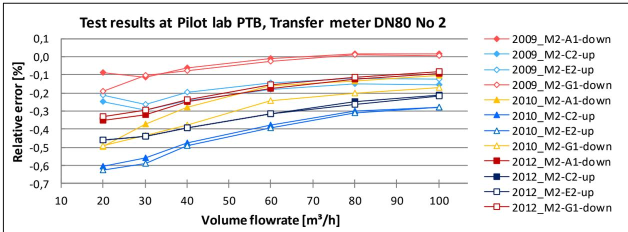
Fig. 16: Turbine flowmeter DN 80 M2 – Measurement error of calibrations at PTB with: M2 - Meter 2 (Turbine flowmeter DN 80)
