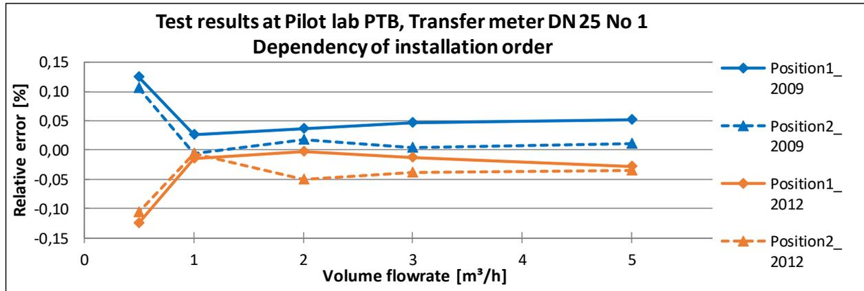
Fig. 9: Turbine flowmeter M1 – Deviation to mean of measurement errors in dependency of installation order (upstream - position 1, downstream - position 2) for comparable measurement conditions (e.g. day 1 to day 3, given as A1/B1 to E2/F2) (see Fig. 2 to Fig. 5)
