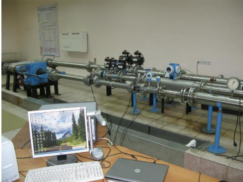
**Picture A.21.** DN80 transfer standard, mounted on standard ГЭТ 63
