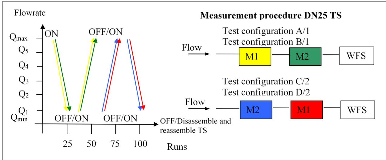
Fig. 2 Measurement procedure A1/B1 and C2/D2 for DN25 transfer standards
