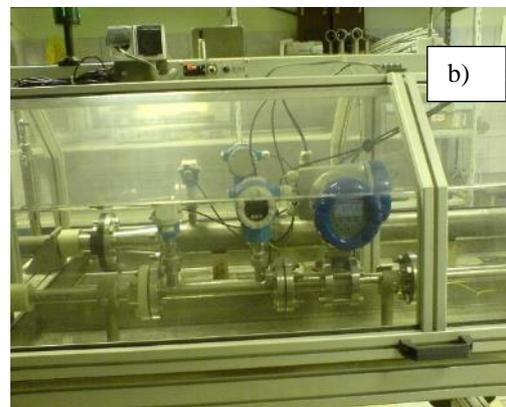
**Figure A.16.** a) Control panel and b) Bench with test lines
