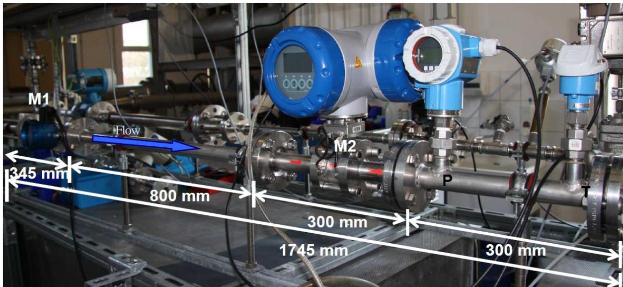
Fig. 7: Photograph of the installed DN25 transfer standards
