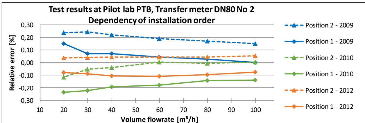
Fig. 18: Turbine flowmeter M2 – Deviation to mean of measurement errors in dependency of installation order (upstream - position 1, downstream - position 2) for comparable measurement conditions (e.g. day 1/4 to day 2/3, given as A1/G1 to C2/E2)
