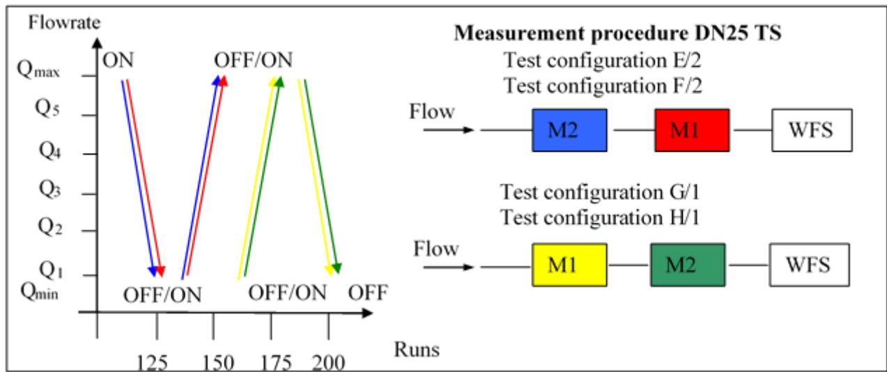
Fig. 3 Measurement procedure E2/F2 and G1/H1 for DN25 transfer standards
