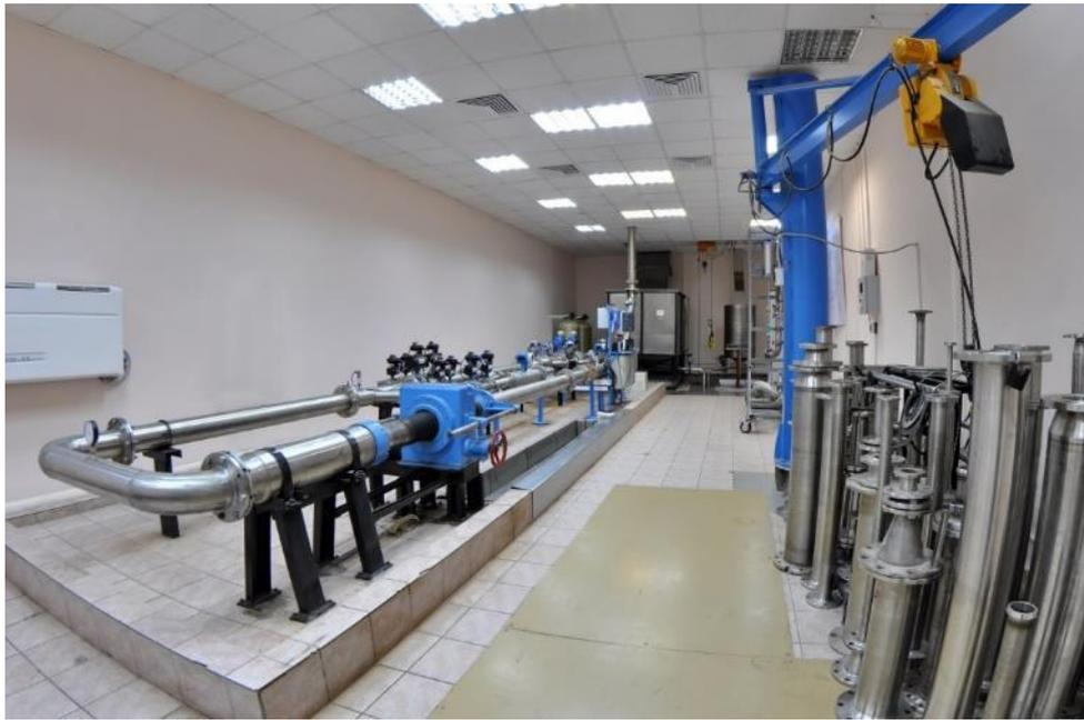
**Picture A.19.** The national primary standard of the unit of mass liquid flow ГЭТ 63
