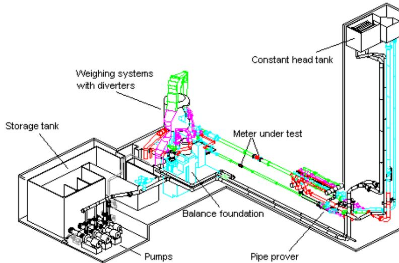
**Figure A.1.** Setup of the Hydrodynamic Test Field (without building)
