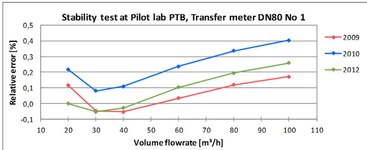
Fig. 19: Turbine flowmeter M1 - Stability of the transfer standard
