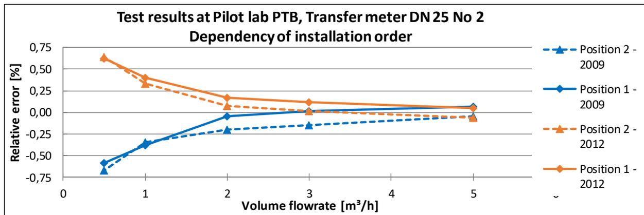
Fig. 12: Electromagnetic flowmeter M2 – Deviation to mean of measurement errors in dependency of installation order (upstream - position 1, downstream - position 2) for comparable measurement conditions (e.g. day 1 to day 3, given as A1/B1 to E2/F2)
