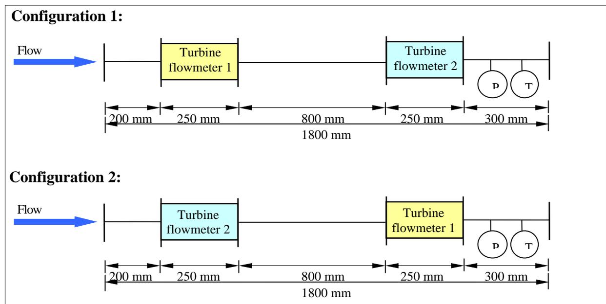
Fig. 13: Measurement configurations 1 and 2 for the DN80 transfer standards
