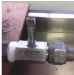
Fig 7. Amplified Pickoff installed on Turbine Meter
