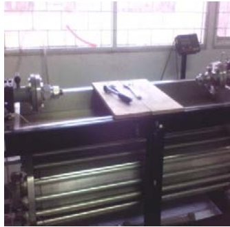
Fig 9. Flanges installed in RCM LIPI Test Bench
