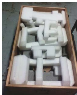
Fig 20. Buffer inside Travelling Box as Protector
