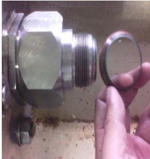
Fig 12. Mechanical Seal in the Flange
