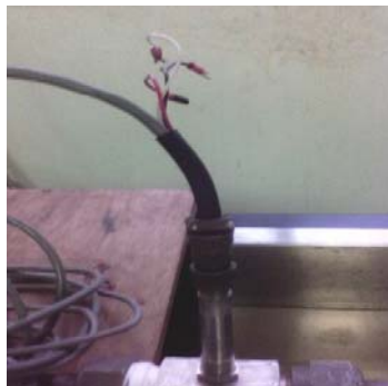
Fig 8. Connector installed on Amplified Pickoff
