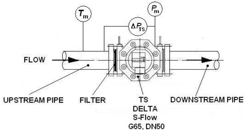
Figure 2 - Recommended installation of the transfer standard
