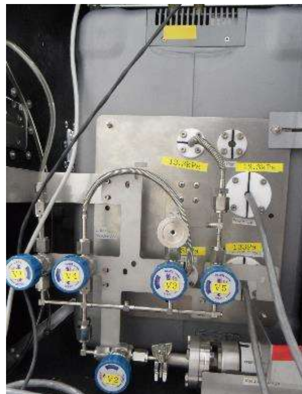
Figure 2. Schematic diagram of the pressure transducer package (PTP).
