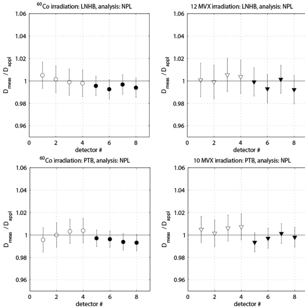
Figure 4. NPL measurement results: Ratio of the dose measured by NPL and the dose stated by LNE-LNHB (top two frames) and by PTB (lower two frames), respectively. Detector # 1:4 corresponds to a nominal dose of 5 Gy whereas detector # 5:8 corresponds to 10 Gy.
