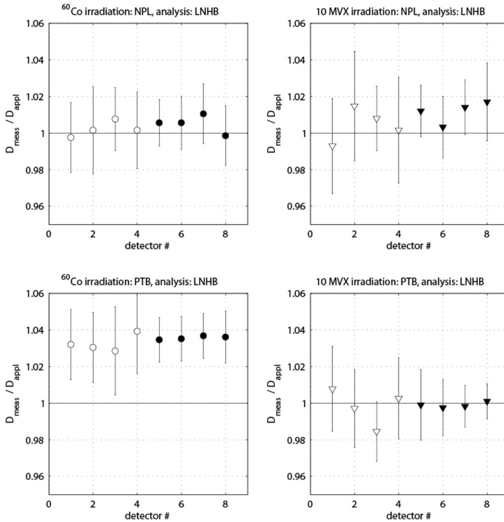
Figure 6. LNHB measurement results: Ratio of the dose measured by LNE-LNHB and the dose stated by NPL (top two frames) and by PTB (lower two frames), respectively. Detector # 1:4 corresponds to a nominal dose of 5 Gy whereas detector # 5:8 corresponds to 10 Gy.
