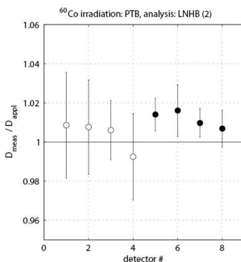
Figure 7. Ratio of the 2<sup>nd</sup> LNHB dose measurement to the stated dose of PTB  $^{60}\text{Co}$  irradiated dosimeters.
