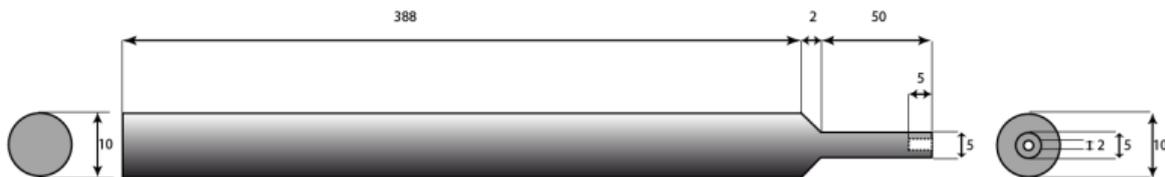
Figure 3. LNE-LNHB positioning system. Dimensions in mm. Not to scale.
