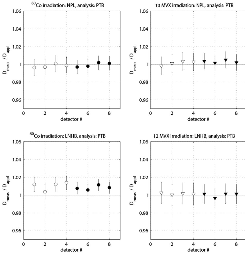
Figure 5. PTB measurement results: Ratio of the dose measured by PTB and the dose stated by NPL (top two frames) and by LNE-LNHB (lower two frames), respectively. Detector # 1:4 corresponds to a nominal dose of 5 Gy whereas detector # 5:8 corresponds to 10 Gy.
