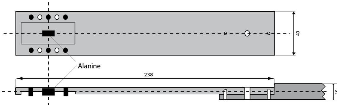
Figure 2. Holder for irradiation of the PTB dosimeters. Dimensions in mm. Not to scale.
