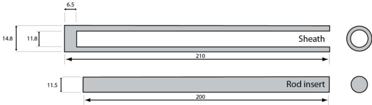
Figure 1. NPL positioning system. Dimensions in mm. Not to scale.
