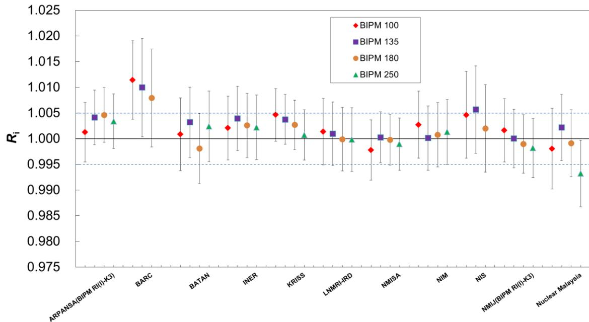
**Figure 7.** The results  $R_i$  for each participating laboratory for the APMP.RI(I)-K3.2013 comparison. Uncertainty bars show the combined standard uncertainty  $u_{R_i}$ . The two linking laboratories (each linked via the other linking laboratory and indicated with brackets) are included for completeness, as are the KRISS and the NIM who each have more recent BIPM.RI(I)-K3 results and hence will not update their degrees of equivalence.
