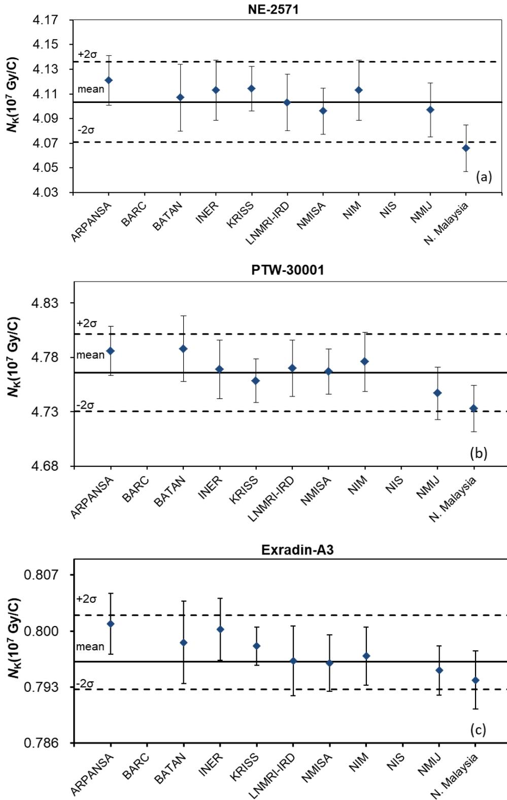
**Figure 6.** Calibration coefficients ( $N_K$ ) of each transfer chamber for BIPM-250 with twice the standard deviation of the distribution indicated, for (a) NE-2571 (S/N 3716), (b) PTW-30001 (S/N 2340) and (c) Exradin-A3 (S/N 143432). The uncertainty bars show the laboratory's reported standard uncertainty  $u(N_K)$ .
