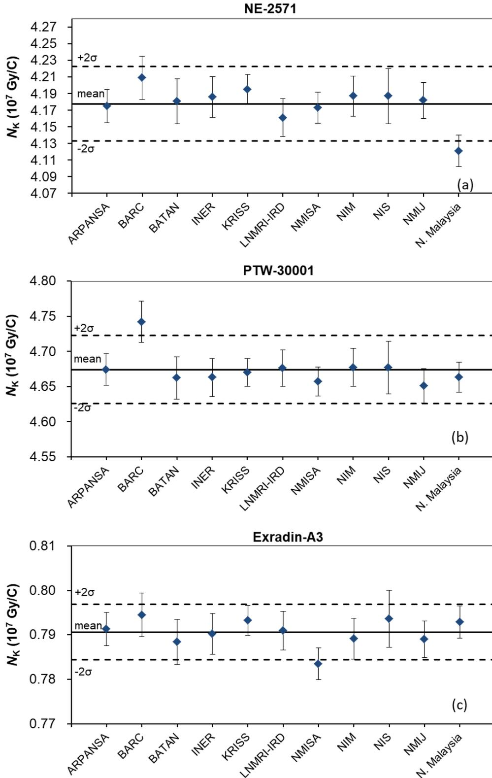
**Figure 3.** Calibration coefficients ( $N_K$ ) of each transfer chamber for BIPM-100 with twice the standard deviation of the distribution indicated, for (a) NE-2571 (S/N 3716), (b) PTW-30001 (S/N 2340) and (c) Exradin-A3 (S/N 143432). The uncertainty bars show the laboratory's reported standard uncertainty  $u(N_K)$ .
