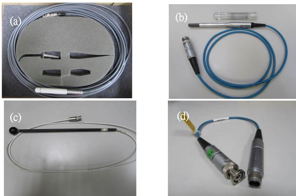
**Figure 1:** (a) NE 2571 chamber (S/N 3716), (b) PTW 30001 chamber (S/N 2340), and (c) EXTRADIN A3 chamber (S/N XR143432), (d) TNC/BNT adaptor
