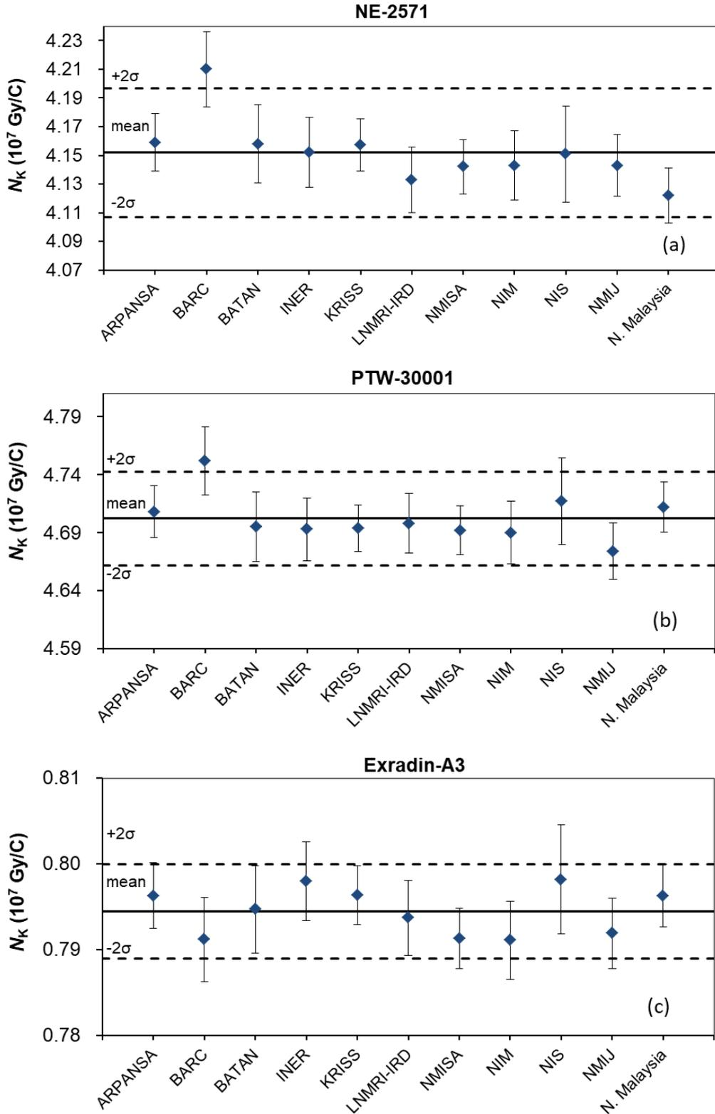
**Figure 4.** Calibration coefficients ( $N_K$ ) of each transfer chamber for BIPM-135 with twice the standard deviation of the distribution indicated, for (a) NE-2571 (S/N 3716), (b) PTW-30001 (S/N 2340) and (c) Exradin-A3 (S/N 143432). The uncertainty bars show the laboratory's reported standard uncertainty  $u(N_K)$ .
