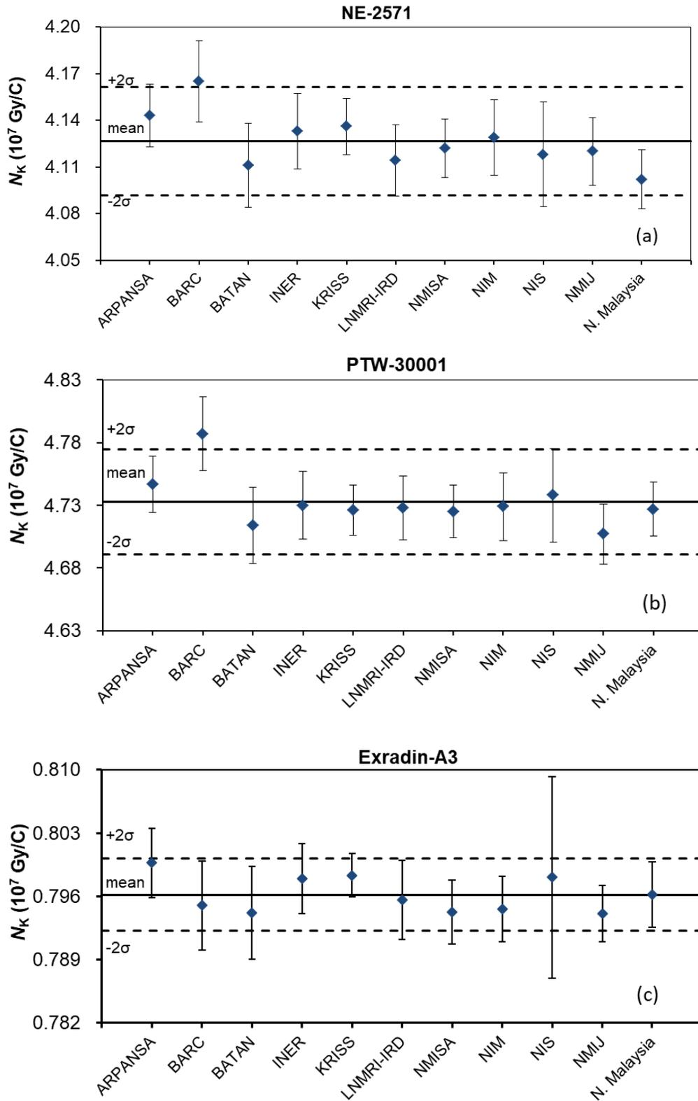
**Figure 5.** Calibration coefficients ( $N_K$ ) of each transfer chamber for BIPM-180 with twice the standard deviation of the distribution indicated, for (a) NE-2571 (S/N 3716), (b) PTW-30001 (S/N 2340) and (c) Exradin-A3 (S/N 143432). The uncertainty bars show the laboratory's reported standard uncertainty  $u(N_K)$ .
