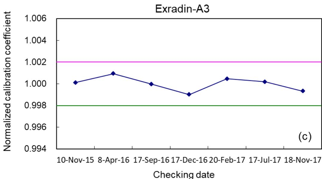
**Figure 2.** Constancy results of transfer chamber measurements made in the  $^{60}\text{Co}$  beam at the INER (a) NE-2571 (S/N 3716) (b) PTW-30001 (S/N 3240) (c) Exradin-A3 (S/N XR143432)
