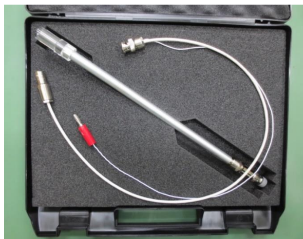
Fig. 2. A photograph of the PTW TN23331 ionization chamber (S/N 0833).
