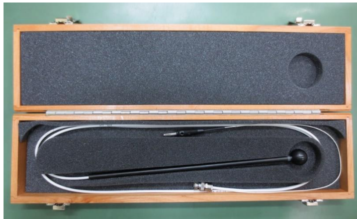
Fig. 1. A photograph of the Exradin A3 ionization chamber (S/N 110).
