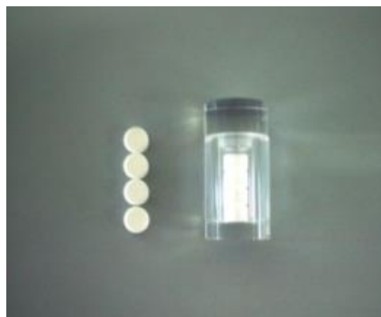
Figure 2. Four alanine pellets were sealed into a cylindrical holder. One holder was used for each irradiation, and each laboratory received 11 holders.
