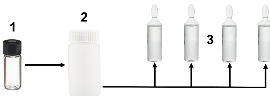
Figure 2: Schematics of dilution. 1 - master solution, 2 - stock solution, 3 - BIPM-SIR ampoules.
