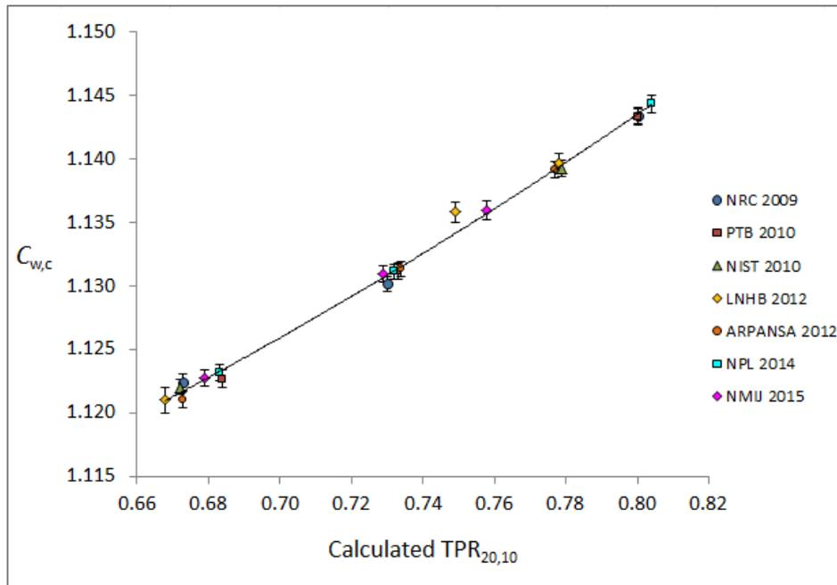
**Figure 1.** The dose conversion factor  $C_{w,c}$  for the BIPM standard, calculated using the phase-space files supplied by participating NMIs. The line is a weighted quadratic fit to the data; the deviations about this line are consistent with the typical statistical standard uncertainty of 5 parts in  $10^4$ .
