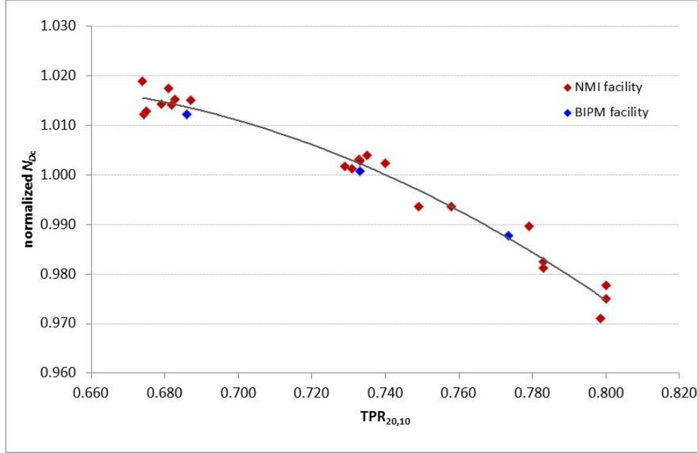
**Figure 2.** The calibration coefficients  $N_{D,c,st}$  determined by the BIPM at various NMI facilities (red) and at the BIPM facility (blue), normalized to the mean, as a function of the measured  $TPR_{20,10}$ . The solid line is a quadratic fit to the combined data set.
