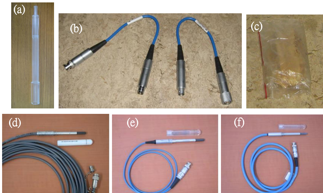
Figure 1: (a) PMMA sleeves made by INER, (b) TNC/BNC adaptors, (c) rubber sheaths which could be used if the PMMA sleeves were incompatible with the laboratory water tank, (d) NE 2571 chamber (S/N 3025, non-waterproof), (e) PTW 30003 chamber (S/N 2340, non-waterproof), and (f) PTW 30013 chamber (S/N 0348, waterproof).
