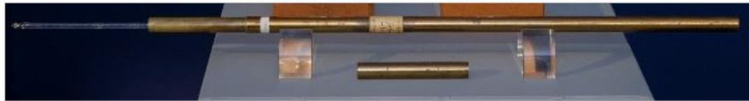
A Tonnelot thermometer was supplied to control the thermal expansion of Pt-Ir.
