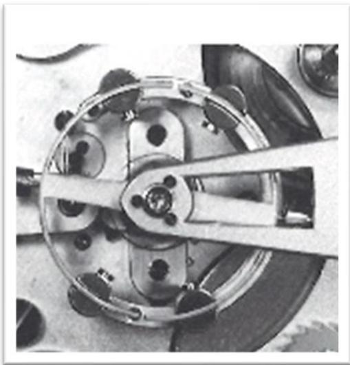
*The integral balance called the Guillaume balance, which eliminates errors due to thermal variations, is used for high-grade watches.*
