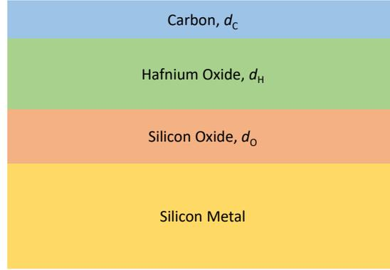
Effective attenuation lengths (EALs) of electrons,  $L$ , are defined for a particular electron energy travelling through a particular material. Thus  $L_{Hf4f,C}$  represents the EAL of Hf 4f electrons in the carbon layer. The ratio of attenuation lengths within a particular material can be calculated with small error. For Al K $\alpha$  radiation equation F-1 and F-2 provide numerical values and associated uncertainties.
