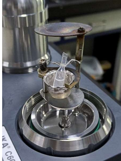
Fig. 1 The photograph of polyethylene capsule containing liquid sample.
